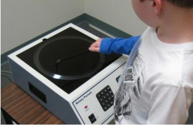
Figure 2. Rotary pursuit tracking device in use.
