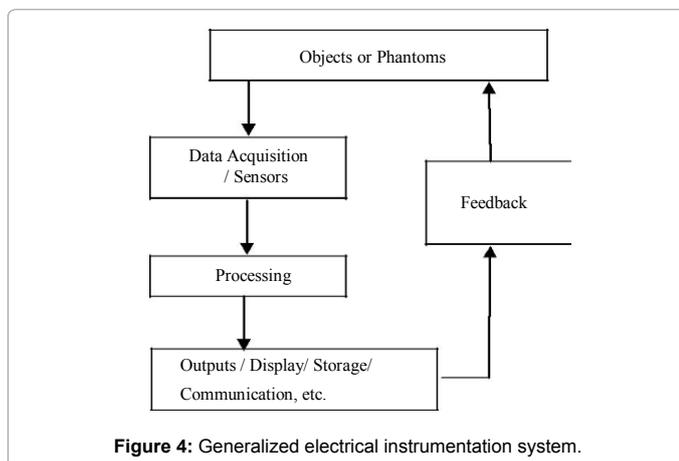
Figure 4: Generalized electrical instrumentation system.
