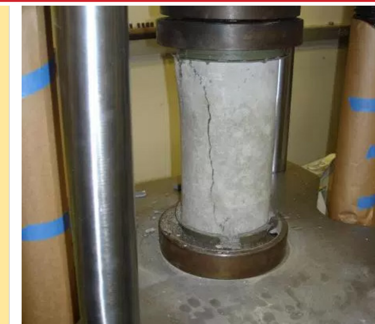
Fig 6: Compression test of a cylindrical sample
