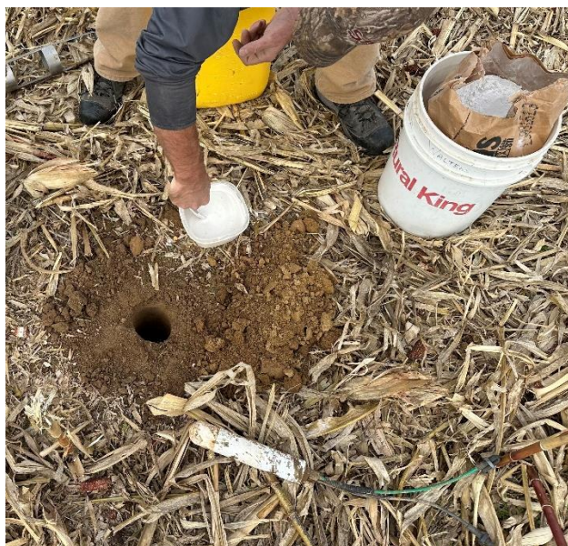
Figure 2.7. Example of tension lysimeter installation with silica flour slurry.
