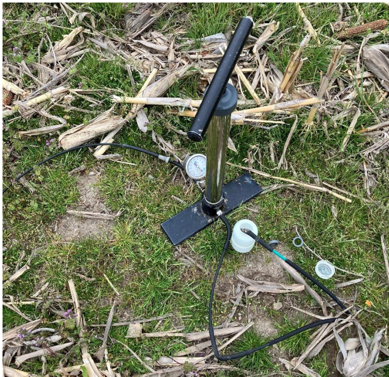
Figure 2.10. Tension lysimeter sampling equipment.
