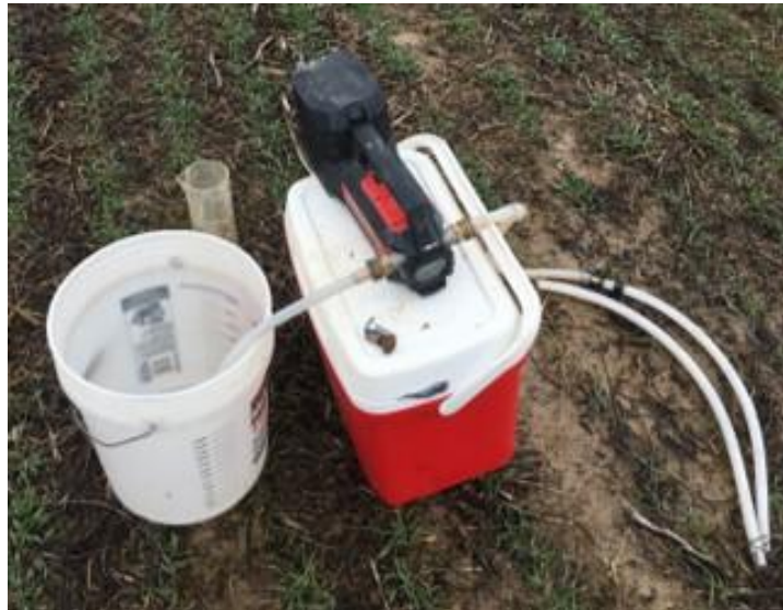
Figure 2.9. Pan lysimeter sampling equipment.
