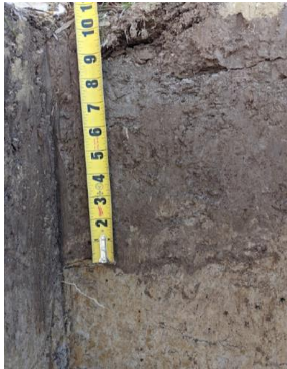
Figure 2.3. Visual indication of A soil horizon and first clay silt loam E horizon used to determine collection pan placement.
