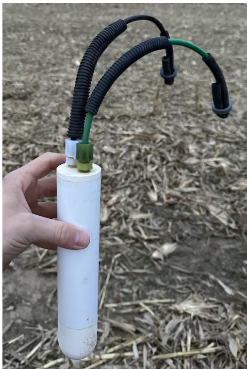
Figure 2.6. Example of the tension lysimeters used.
