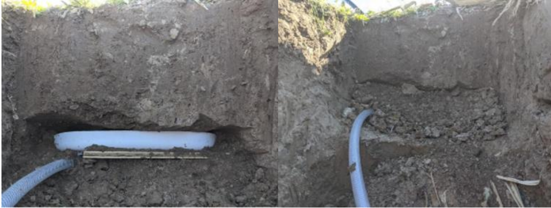
Fig. 2.4. Pan lysimeter collection plate placement in a research plot (left) and after being backfilled (right).
