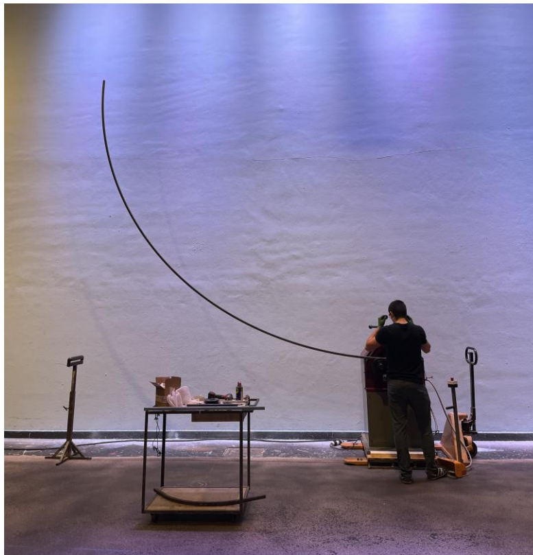
Figure 3.3 – Uriel bending 1” box tube with the new roller bender – Property of author
