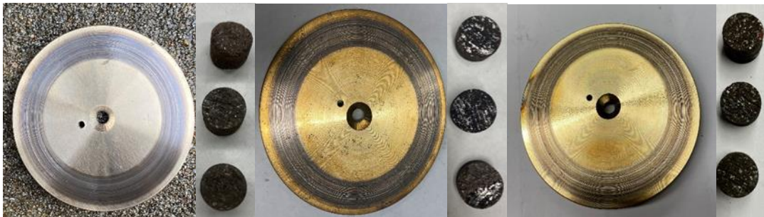
Figure 19: 3D printed SS316 rotor and laboratory-formulated NAO pad samples
