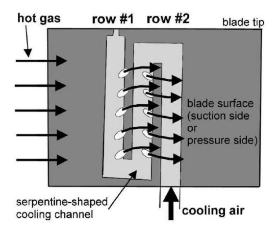
Figure 7. Application of the DJFC to a cooled GT blade (schematic drawing) [8]
