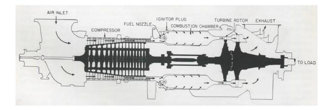
Figure 1 Air flow diagram of the 4,500-horsepower gas turbine engine out of a locomotive. Exhaust gases expelled through the roof aperture at velocity of 150 m.p.h., 850° F with volume of 150,000 cubic feet. [1]
