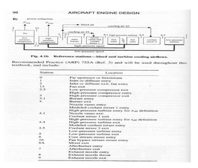
Figure 8. Bleed & turbine cooling airflows diagram, key [9]
