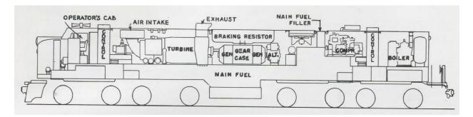
Figure 2 Cutaway side view of the 4,500-horsepower gas turbine electric locomotive shows the layout of the interior equipment while showing the exterior layout of 7,200-gallon fuel formed structural base, carbody rested on two span bolters containing two four-wheel powered trucks.[1]
