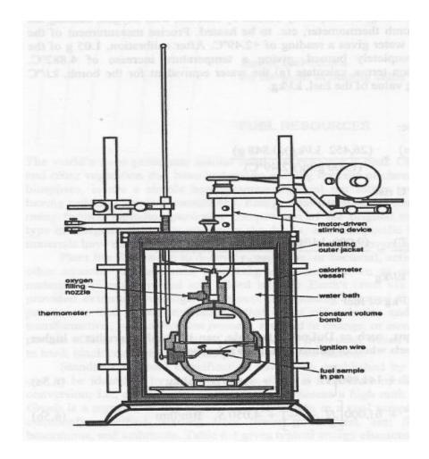
Figure 5 Constant-volume oxygen bomb calorimetry diagram [5]
