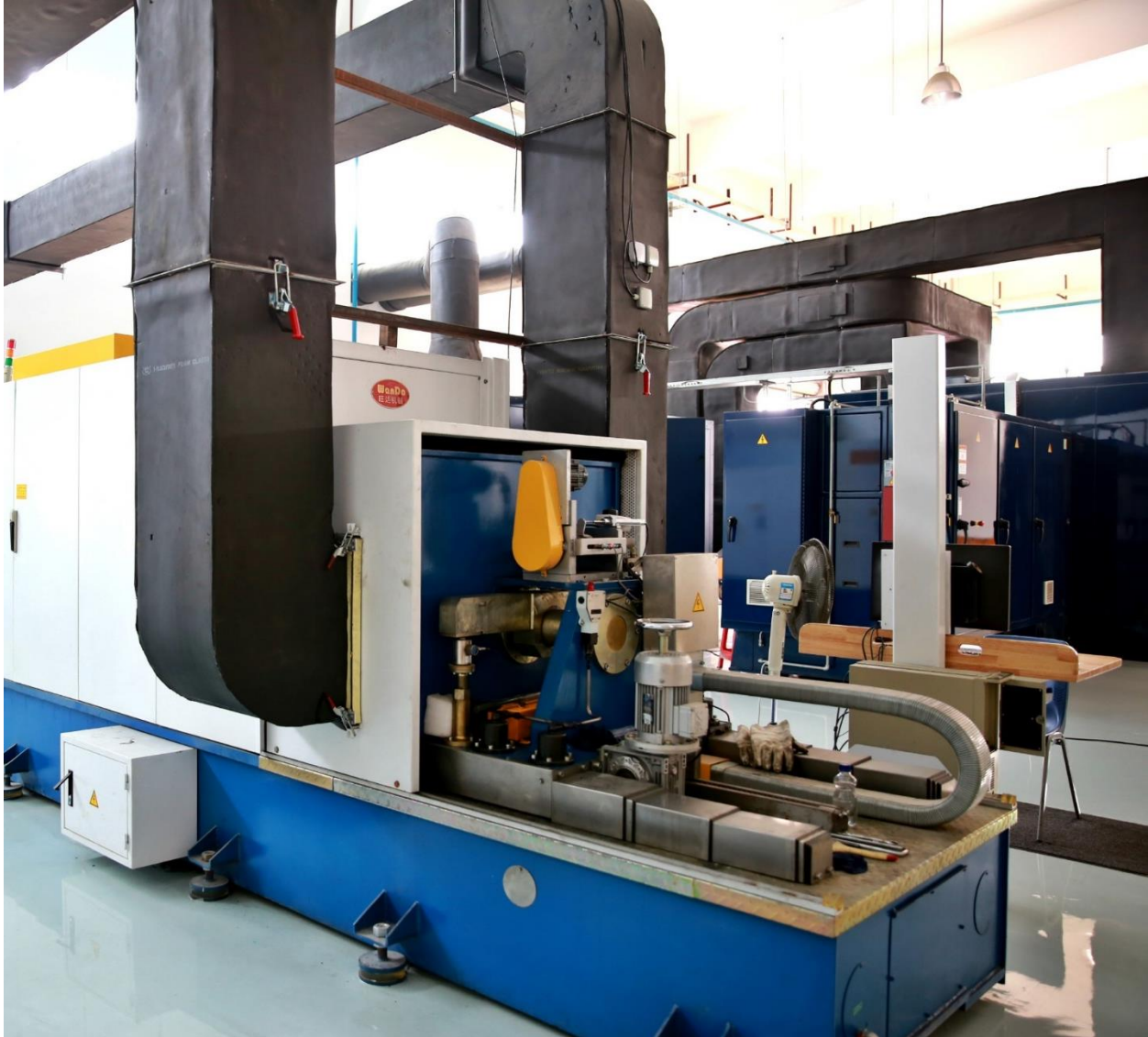
Figure 4: Picture of full scale automotive brake dynamometer (source: asimcoglobal.com)
