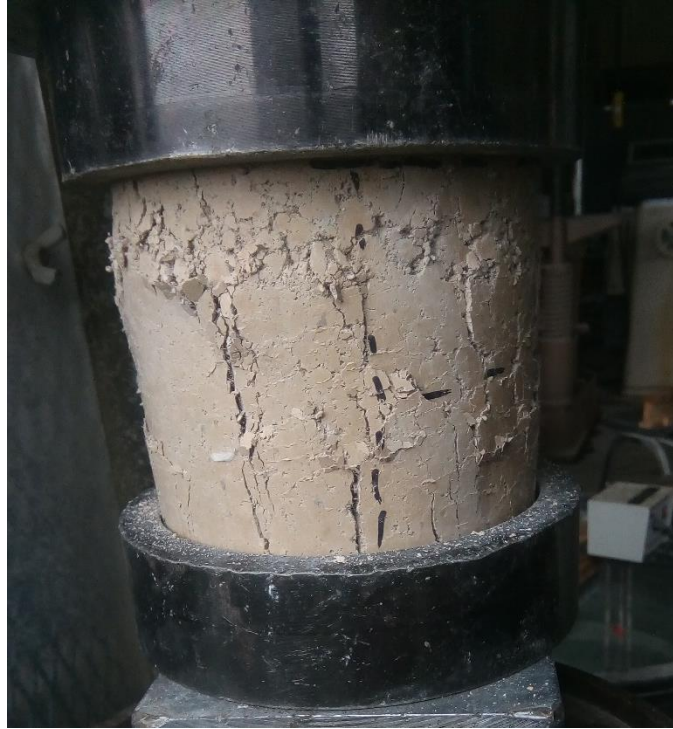
Figure F-11: EPK sample with cement + fiber during compression test, improves the brittle failure pattern
