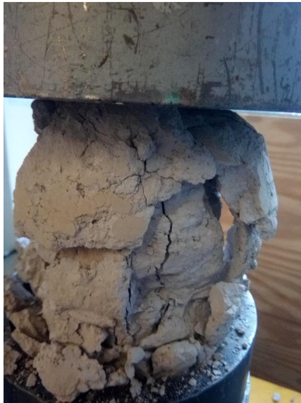
Figure F-10: EPK sample with cement only (without fiber) crumbled completely during compression test
