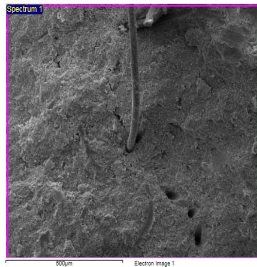
Figure 4-10: EDAX result of EPK clay mixed with 5% cement and 0.5% fiber
