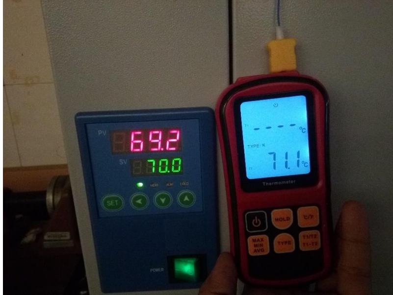
Figure F-1: Drying Temperature setup for Wetting-Drying Test
