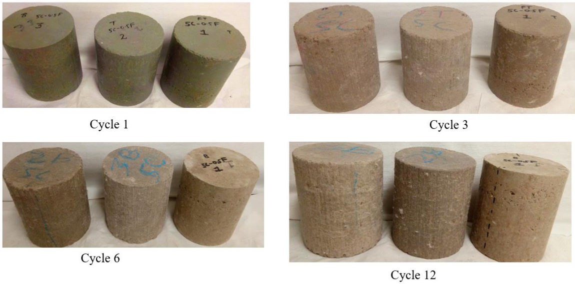
Figure 4-43: Various stage of freezing-thawing test of FT_5C_0.5F
