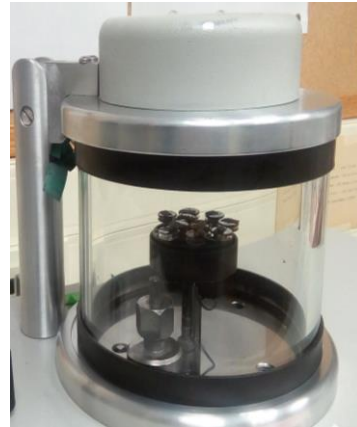
Figure 3-13: Sample Coating with Au/Pd
