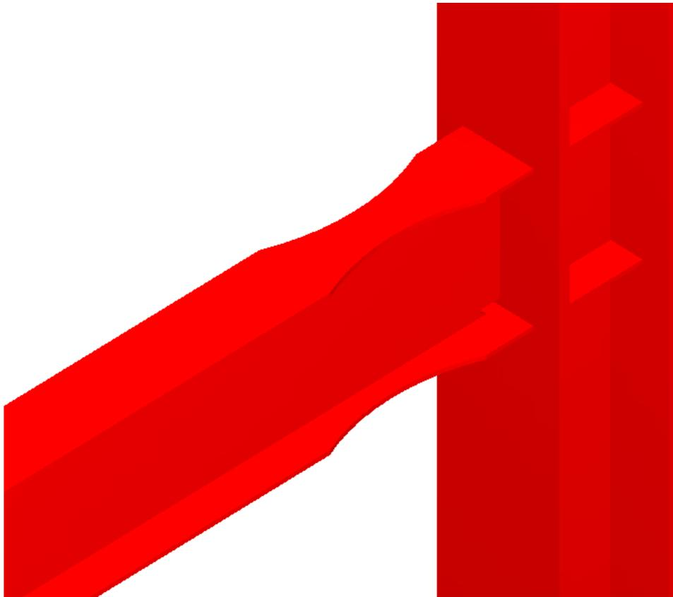
Figure 2.4.2 Typical Reduced Beam Section Connection
