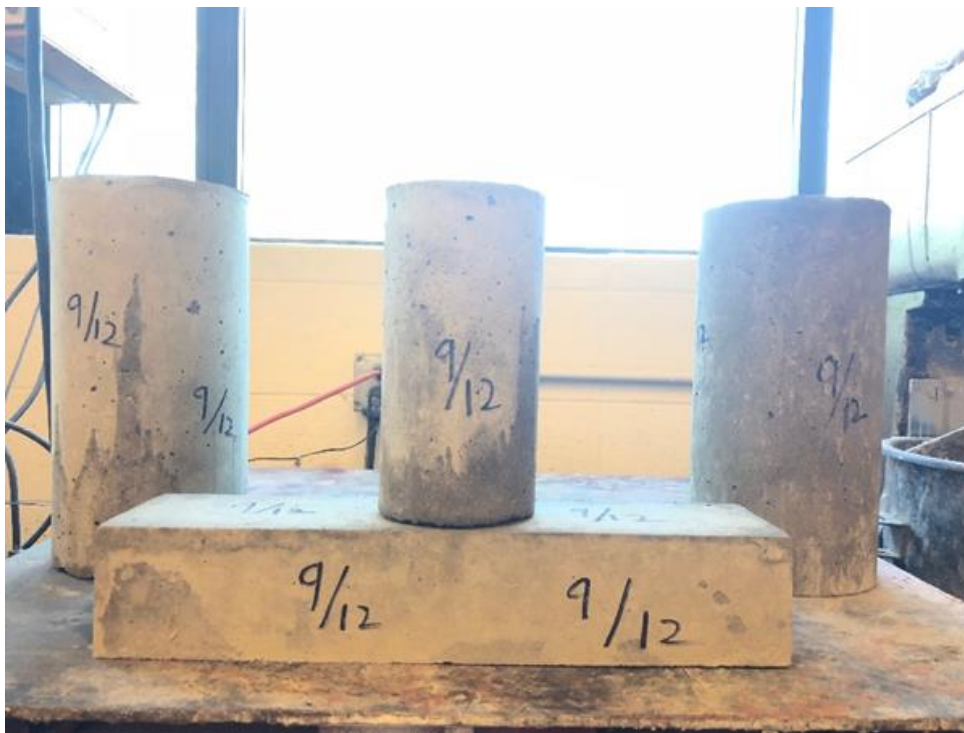
Figure 31. Concrete samples with different shapes and sizes
