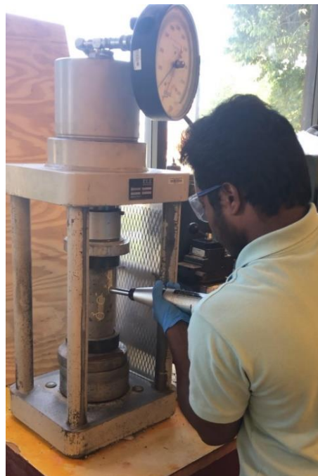
Figure 20. Rebound hammer test on concrete cylinder
