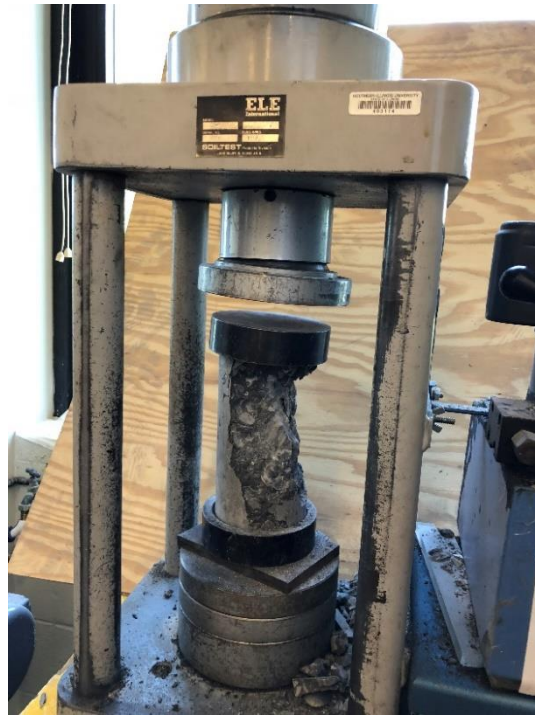
Figure 21. Concrete cylinder crushed for compressive strength
