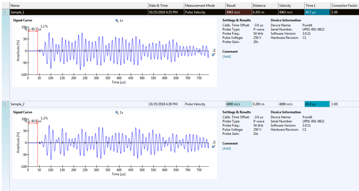
Figure 32. P-wave velocity measurements on Sample (1 & 2) from batch-1 of 6000 psi
