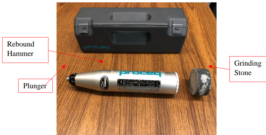
Figure 19. Rebound hammer testing equipment
