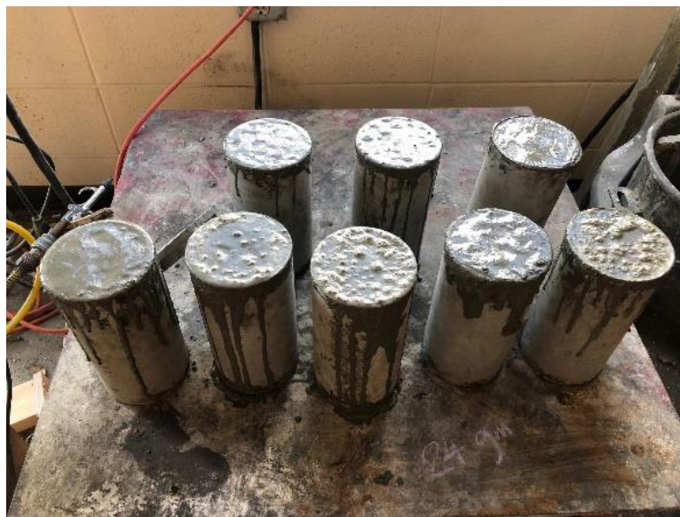
Figure 13. Molded cylinders placed on vibratory table
