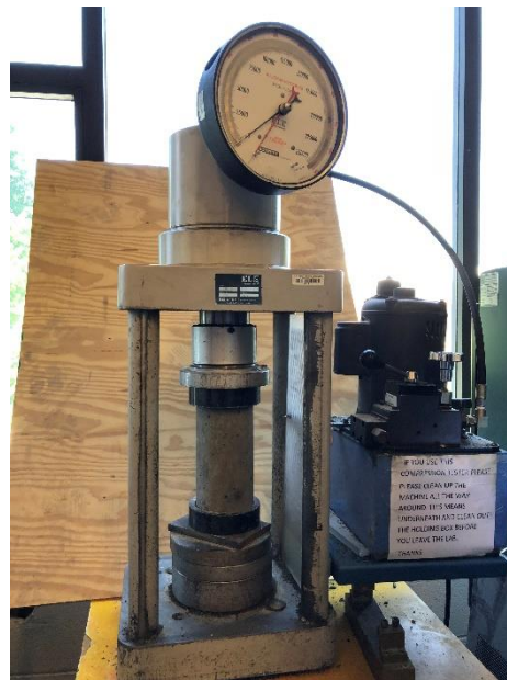
Figure 11. Compressive strength testing of concrete cylinder
