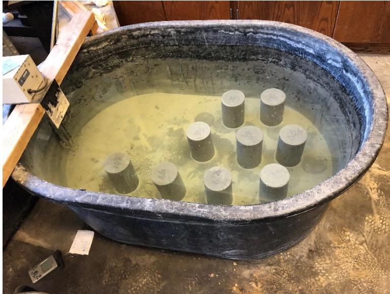
Figure 14. Curing the samples in water
