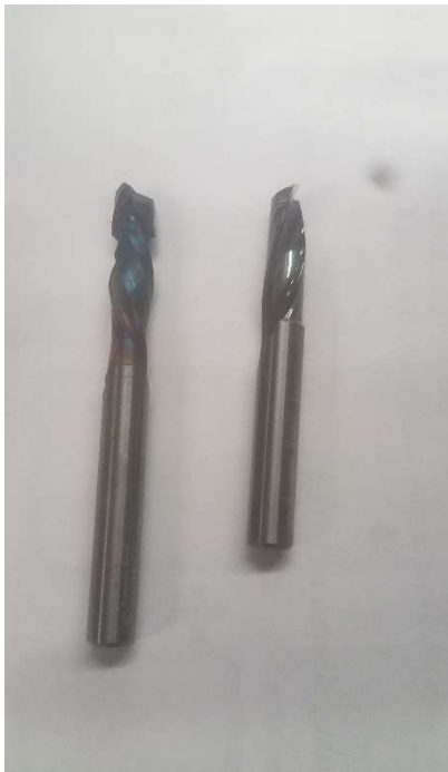
Figure 7 - (Right) Spiral O-Flute Bit vs (Left) Compression Bit – Property of Author
