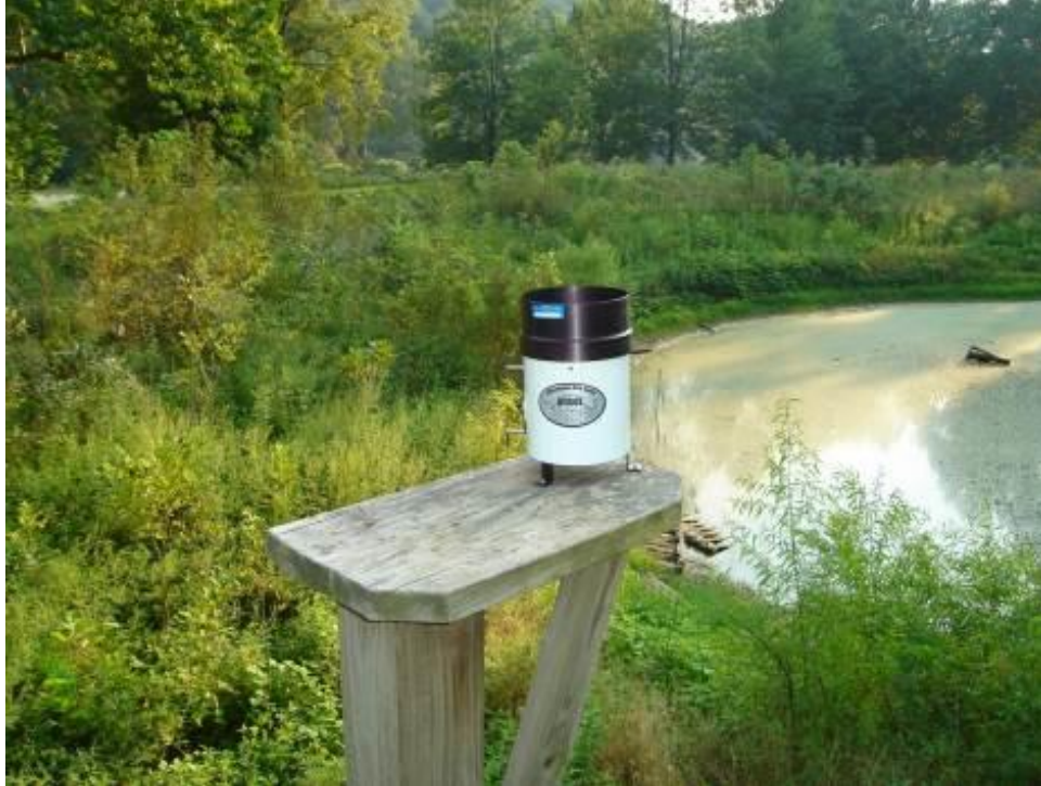
Photograph 3-1. Tipping bucket rain gauge that was installed at the TTSF study location to provide site specific precipitation data.
