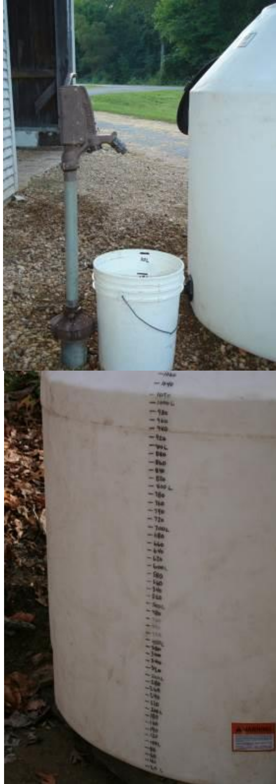
Photograph 3-4. Tanks were pre calibrated and labeled every 20 L to ensure accurate volume totals per storm event.
