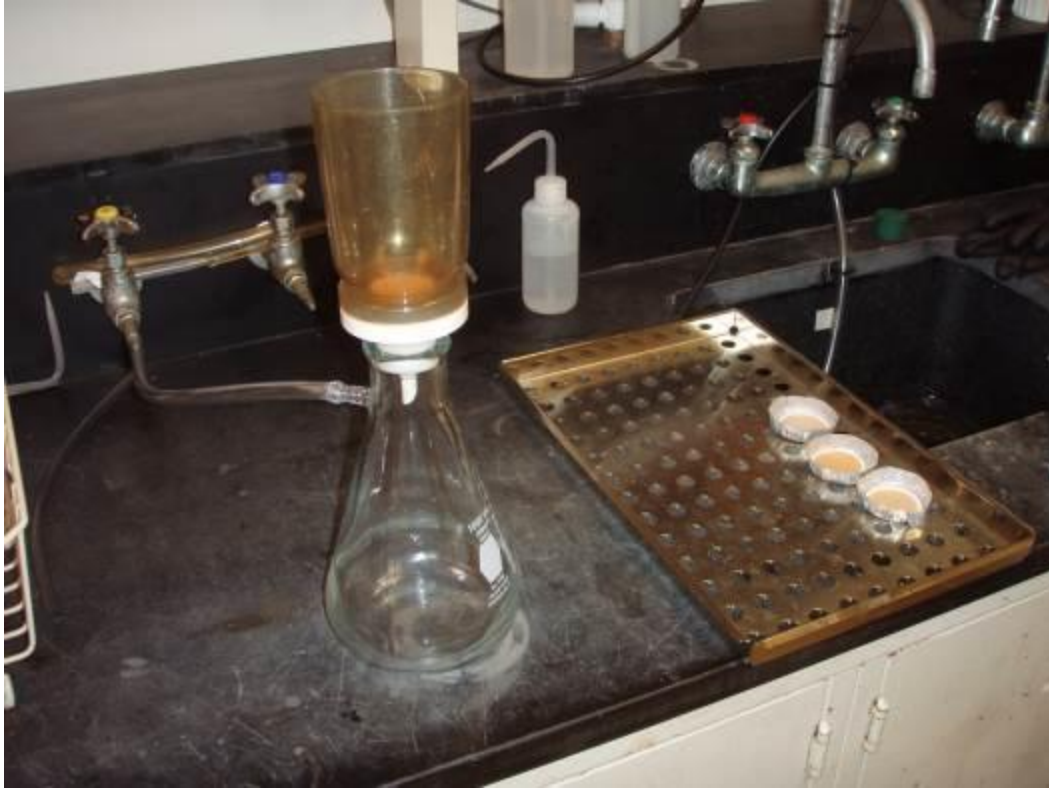
Photograph 3-11. Water samples were suction filtered through a Whatman glass microfiber filter to separate the total residue non-filterable suspended solids from the water.
