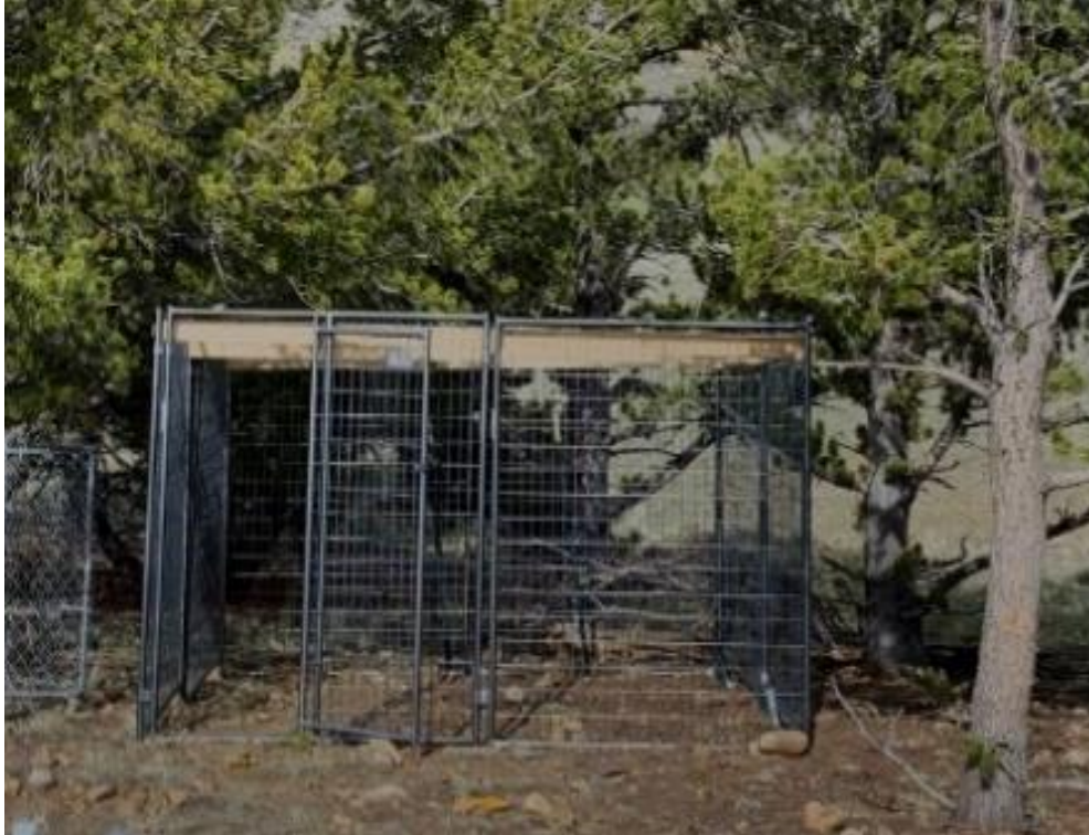
Figure 3-1: 3m x 3m five-panel galvanized steel cage anchored by scavenger deterrent panels.
