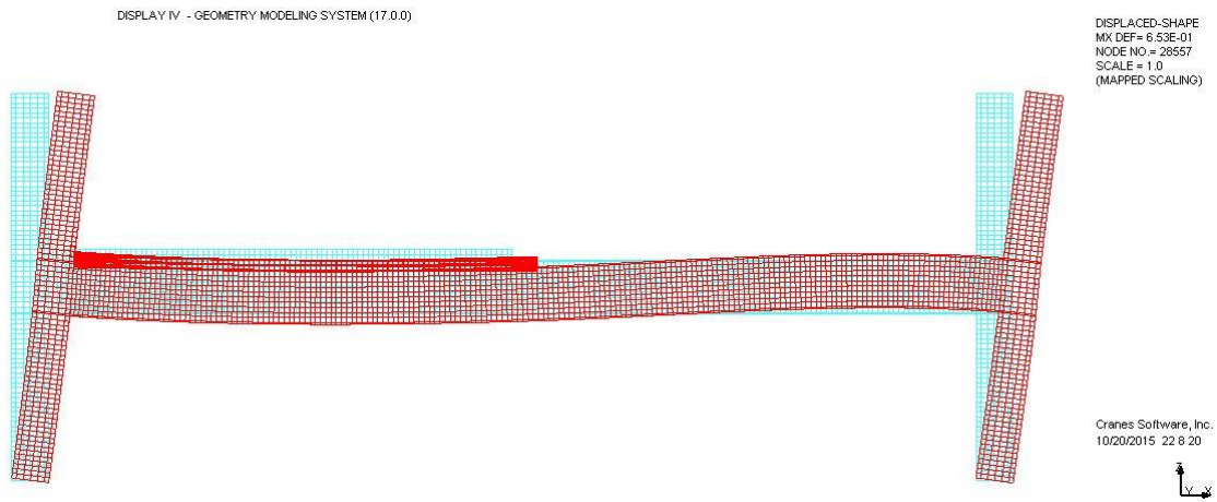
Figure B.22: Elastic deformation (Model 1b)
