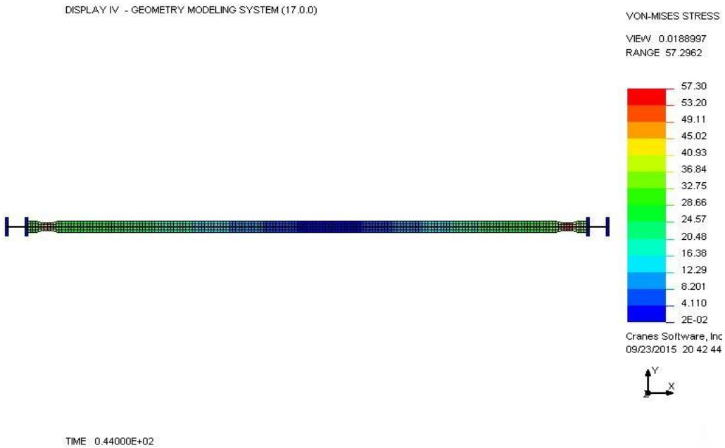
Figure B.2: Von-Mises stress top view (Model 1a)
