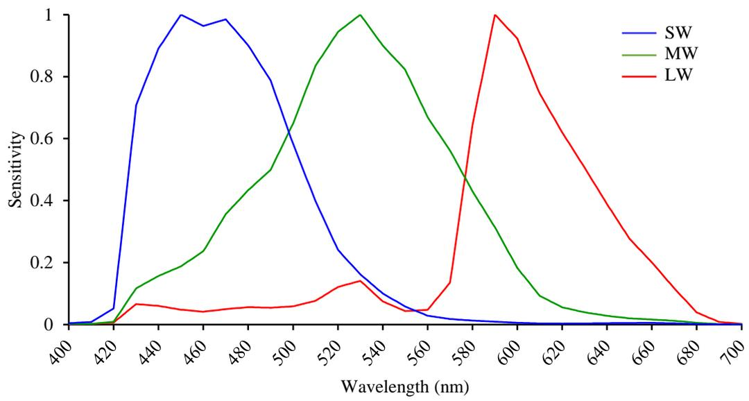
Figure 6.3 Spectral sensitivity of the short (SW), medium (MW), and long (LW) wave receptors for a Nikon D5200 (data from Jiang et al., 2013).
