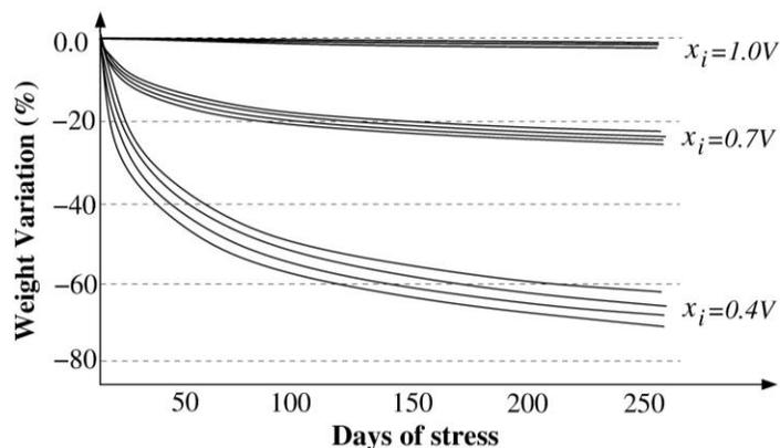
Figure 5.6. The weights change due to transistor aging for various input voltage  $x_i$ .
