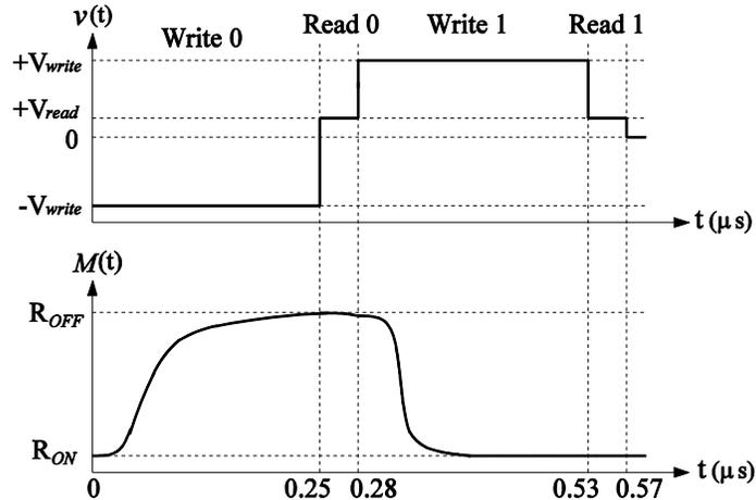
Figure 2.2. Resistivity behavior for all four operations ( $w0$ ,  $w1$ ,  $r0$ , and  $r1$ ) during test for a bipolar metal-oxide memristor with  $R_{ON}=100\Omega$ ,  $R_{OFF}=100K\Omega$ ,  $V_{write} = 3.3V$ ,  $V_{read} = 0.8V$ , using [15, 35].
