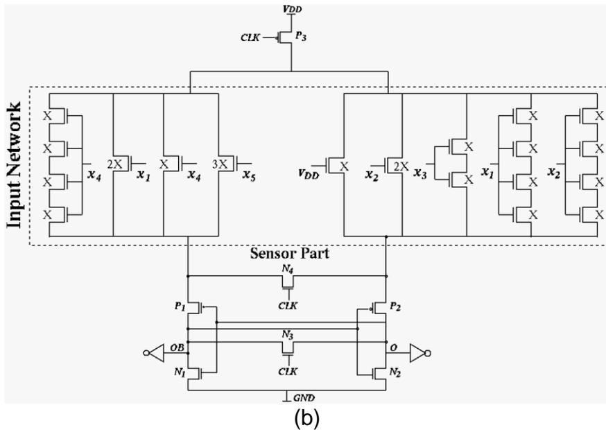
Figure 3.2. The CTG implementation for function  $F_2$  in example 3 when using (a) integer weights [53] (b) rational 1-weights with value  $w_j$ , for when  $1 \leq j \leq l$  and  $l = 4$ .
