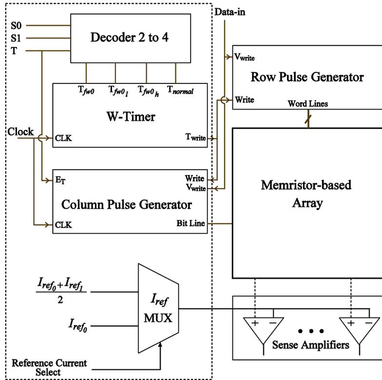
Figure 2.11. Schematic of the proposed USF DfT.
