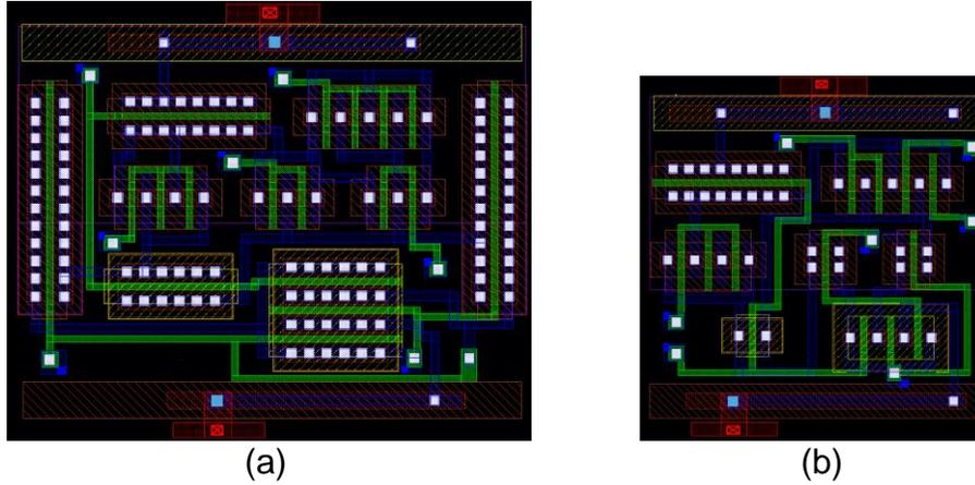
Figure 3.6. (a) The layout for 1-CTG implementation of function  $[w_1, w_2, w_3; w_T] = [4, 2, 2; 3]$  as in [53] (b) the layout of the same function implemented using rational weights  $[w_1^1, w_2^1, w_3^1; w_T^1, w_T^2] = [2, 1, 1; 1, 1]$ .
