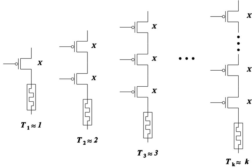
Figure 4.3. Memristive  $m$ -weight components for  $1 \leq m \leq k$ .
