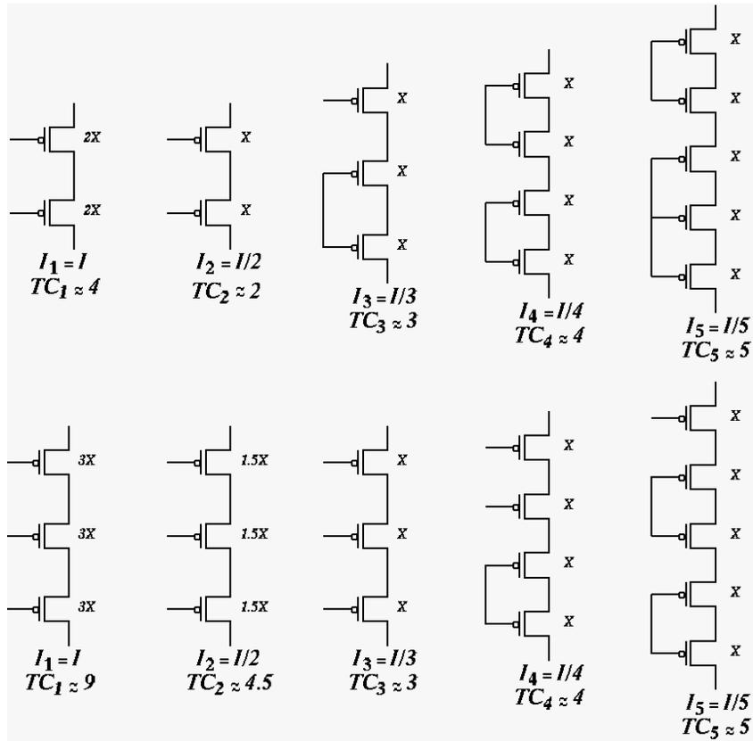
Figure 3.5. Rational  $k$ -weights components with values  $1/j$  for  $2 \leq k \leq 3$  and  $1 \leq j \leq 5$ .
