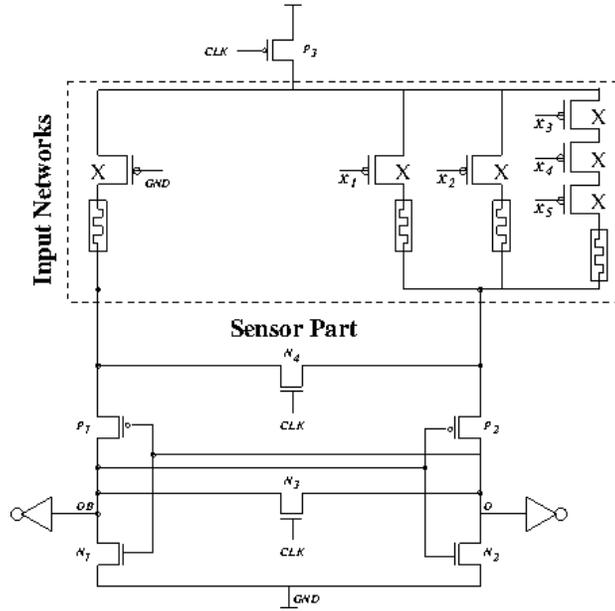
Figure 4.4. The memristive Current mode TG (CTG) implementations for function  $F_3$  in example 3.
