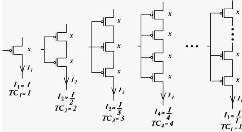
Figure 3.1. 1<sup>st</sup>-order components that implement rational 1-weights with value  $1/j$ , for  $1 \leq j \leq l$ .
