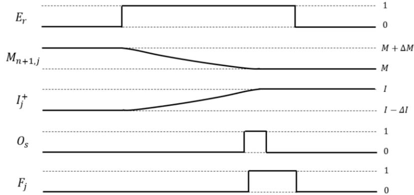
Figure 5.4. Timing diagram for signals  $E_r$ ,  $O_s$ , and  $F_j$  during the restore operation for target column  $C_j^+$ .
