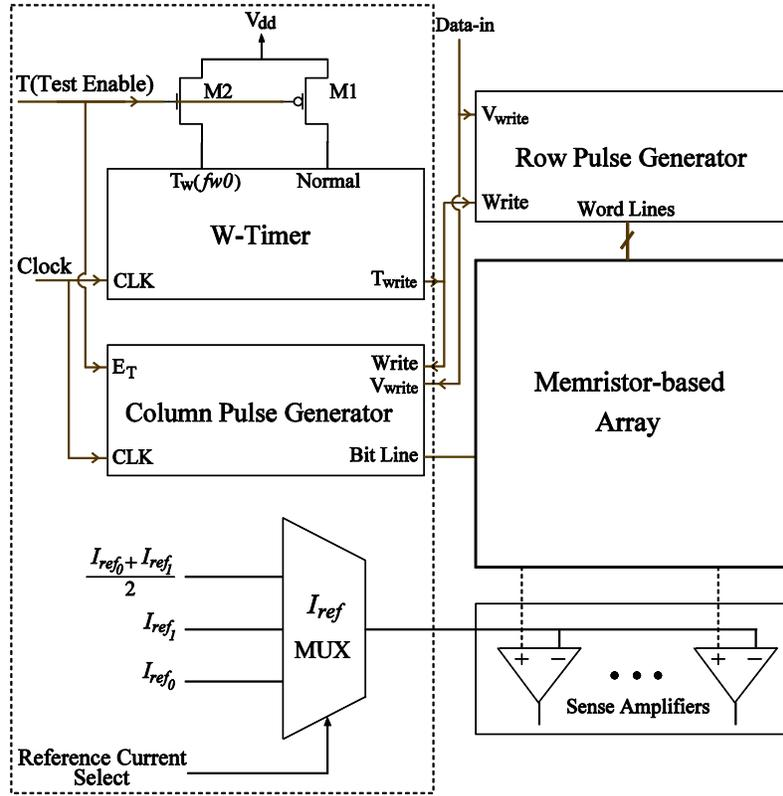
Figure 2.9. Schematic of the proposed DfT.
