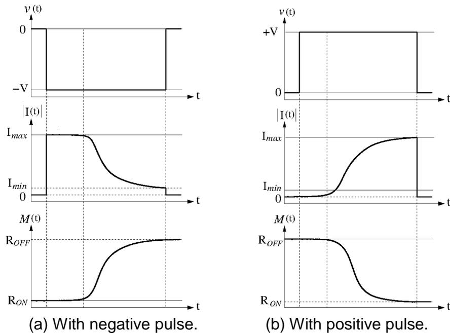
Figure 4.1. Resistivity and current behavior for positive and negative writes for a bipolar metal-oxide memristor with  $R_{ON}=5K\Omega$ ,  $R_{OFF}=5M\Omega$ ,  $\pm V = 1V$ , using [15, 94].
