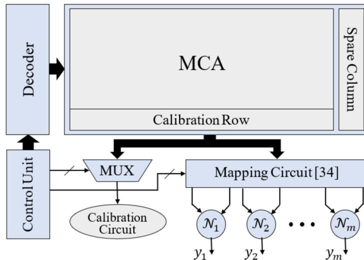
Figure 5.2. Enhanced ANN architecture including control and mapping unit for isolating the target column.
