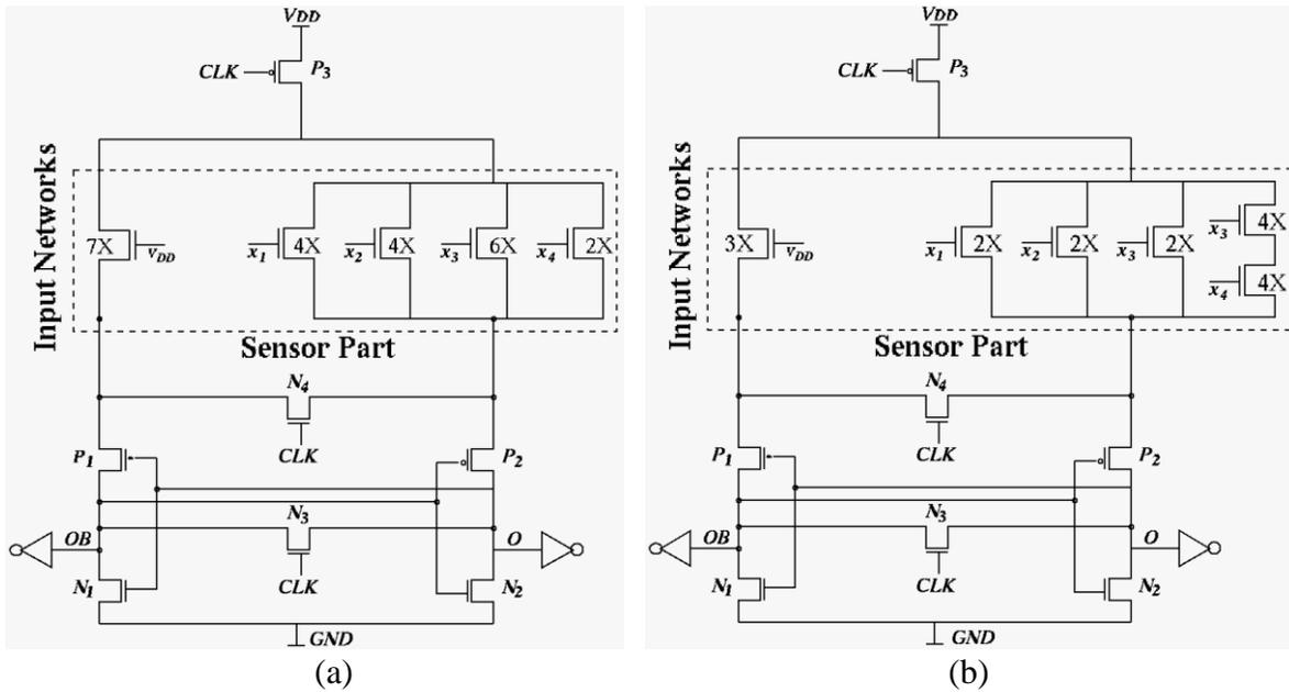
Figure 3.4. The CTG implementation for function  $F_6 = x_4x_3 + x_3x_2 + x_3x_1 + x_2x_1$  with (a) 1-CTG as 1-TF [53] (b) proposed 2-CTG as 2-TF [82].
