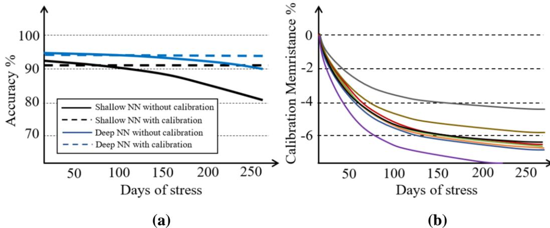
Figure 5.7 (a) The accuracy over days of stress of the implemented shallow and deep neural networks with and without using the built-in calibration circuit, and (b) calibration memristance for each column in output layer over days of stress to compensate the aging effect.
