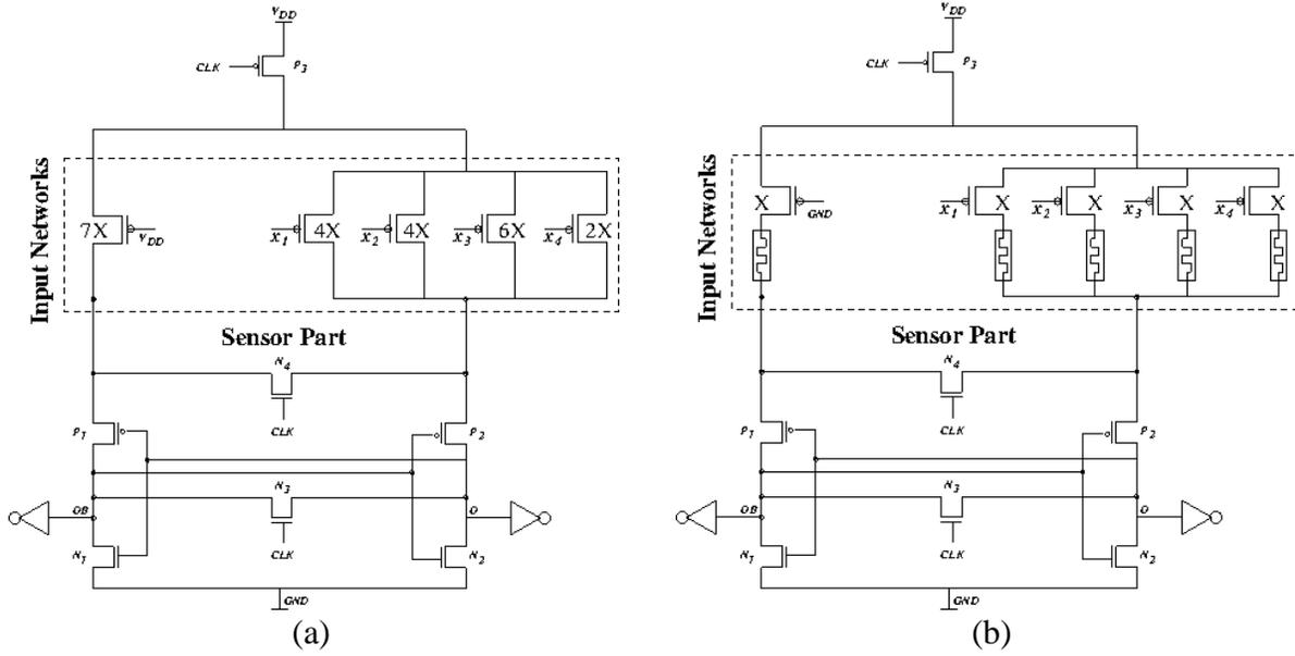
Figure 4.2. The Current mode TG (CTG) implementations for function  $F_2$  in example 2 (a) CTG as in [52] (b) memristive CTG as in [76].
