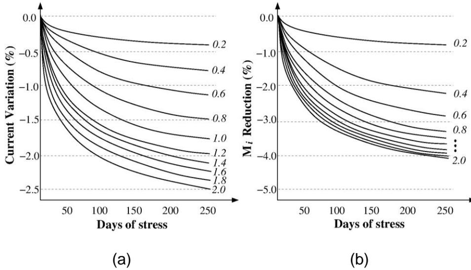
Figure 5.5. (a) The current degradation over time due to aging, and (b) the calibration resistivity  $M_j$  changes over time to compensate the current degradation. Ten different weight values are considered.
