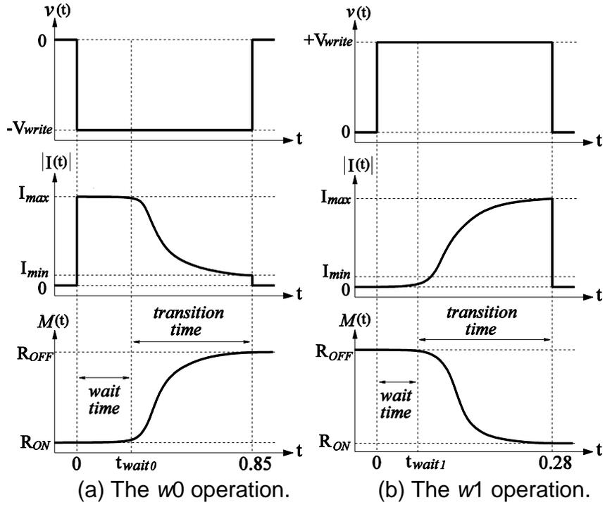
Figure 2.1. Resistivity and current behavior for writes in the normal mode of operation for a bipolar metal-oxide memristor with  $R_{ON}=100\Omega$ ,  $R_{OFF}=100K\Omega$ ,  $V_{write} = 1.2V$ ,  $V_{read} = 0.8V$ , using [15, 35].
