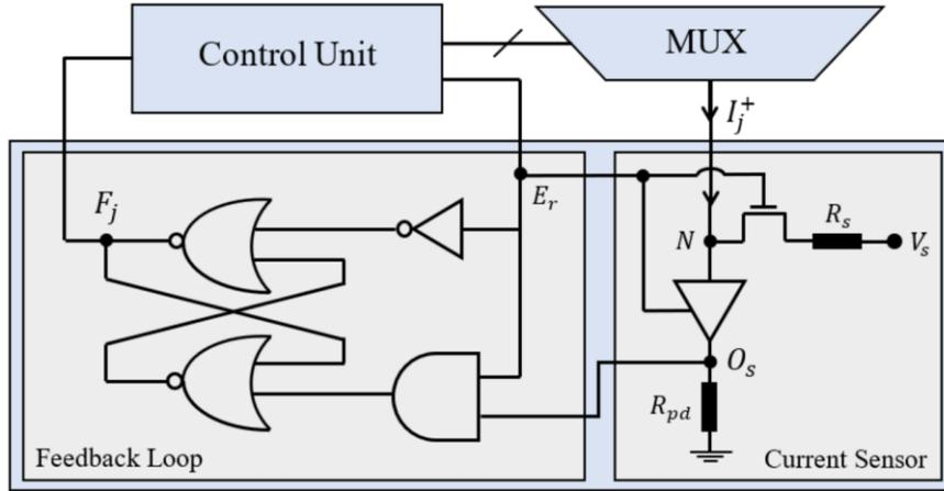
Figure 5.3. The circuitry of the proposed current-based calibration circuit.
