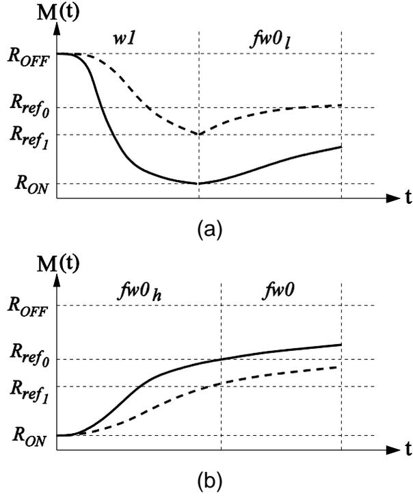
Figure 2.7. Simulation results for the fault free and faulty cell with (a) USF1 and (b) USF0.
