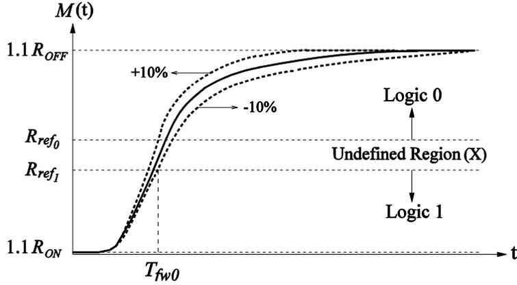
Figure 2.6. The undefined state for a memristor cell, and the value of  $T_{fw0}$  considering 10% doping variation. The memristor also suffers from 10% increment in size ( $L/A$ ).
