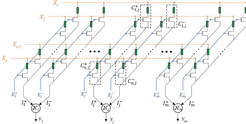
Figure 5.1. Memristive crossbar array for feedforward NN as in [126] and the interface modules.
