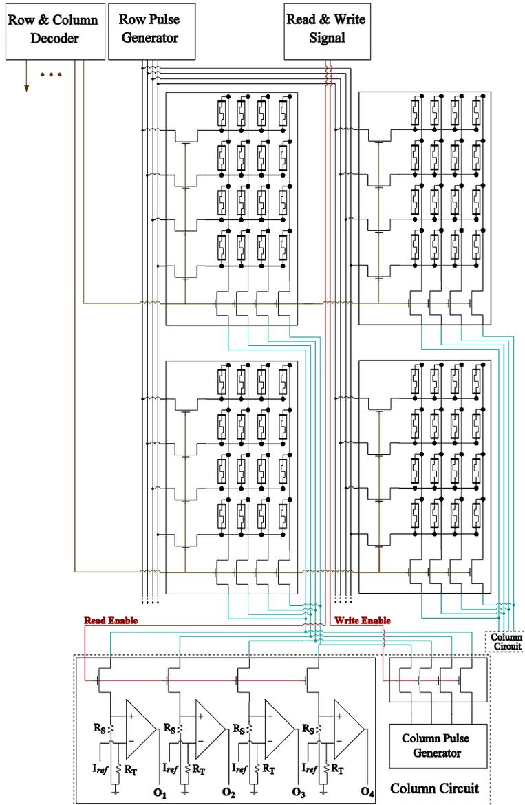
Figure 2.3. Hybrid crossbar architecture using the combination of memristor and isolating transistor [3, 28].
