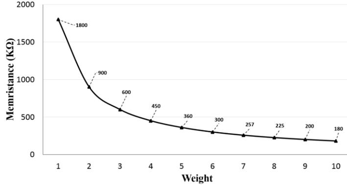
Figure 4.5. Different resistivity values to implement memristive  $k$ -weights with value  $w$ , for  $1 \leq w \leq 10$  and  $1 \leq k \leq 4$ .
