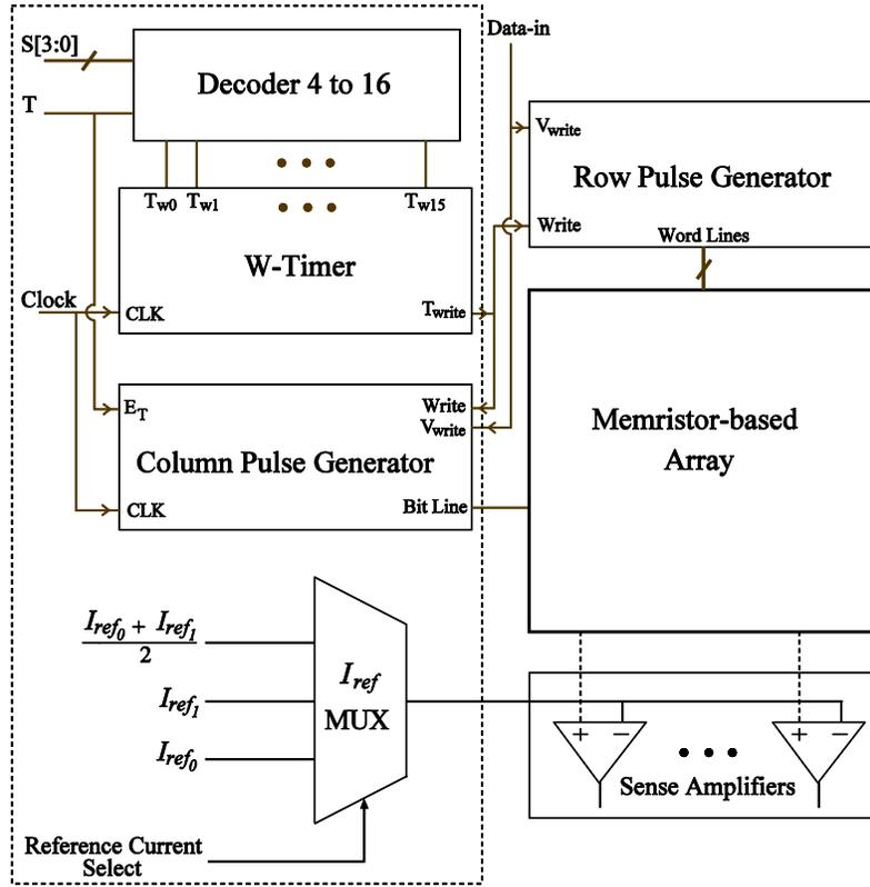
Figure 2.10. Schematic of the proposed programmable DfT.
