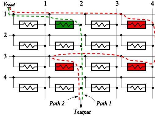
Figure 2.8. Sneak-path testing in a 4x4 high density crossbar memory.
