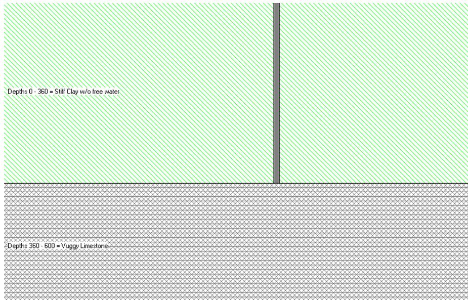
*Figure 2.9* End-bearing straight pile in stiff clay case
