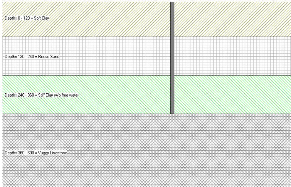
*Figure 2.11* End-bearing straight pile in three layers of soil case
