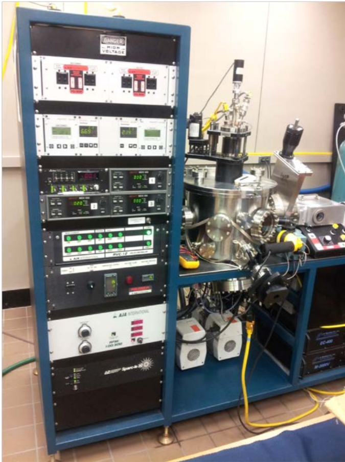
Figure 2.2 The unbalanced magnetron sputtering machine used for most of the depositions, colloquially known as “Maggie”.
