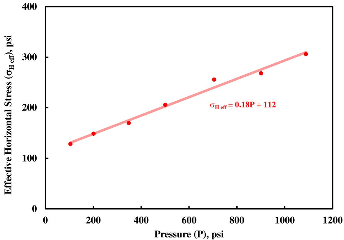
Figure 4-4: Variation in effective horizontal stress with methane depletion
