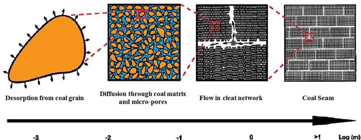
Figure 1-1. Gas transport mechanisms in a coalbed reservoir (Srivastava, 2005)
