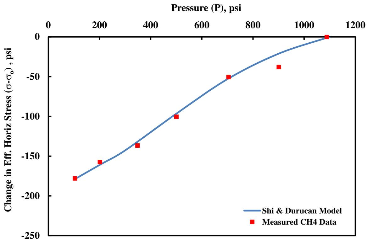
Figure 4-7: Measured and modeled change in eff. horizontal stress with methane depletion (Variable E)
