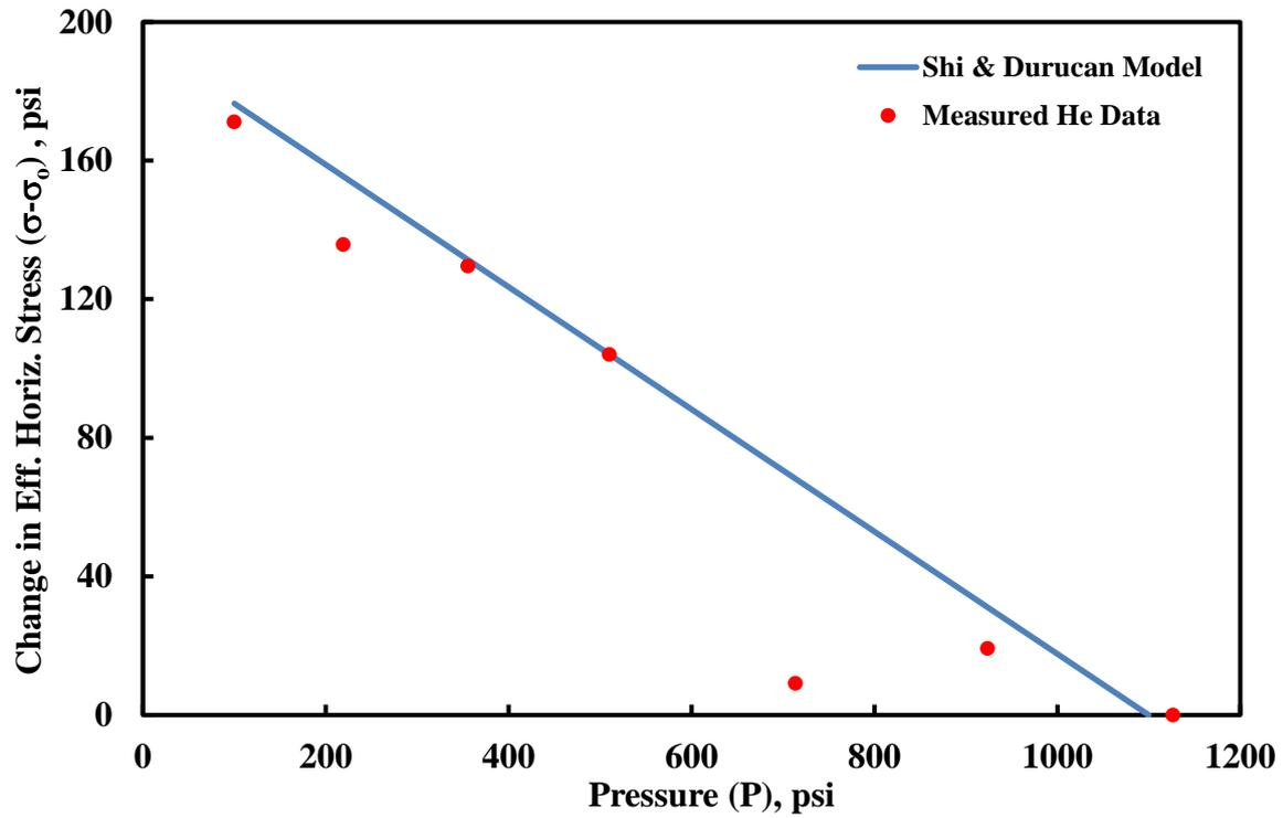
Figure 4-5: Measured and modeled change in effective horizontal stress with helium depletion
