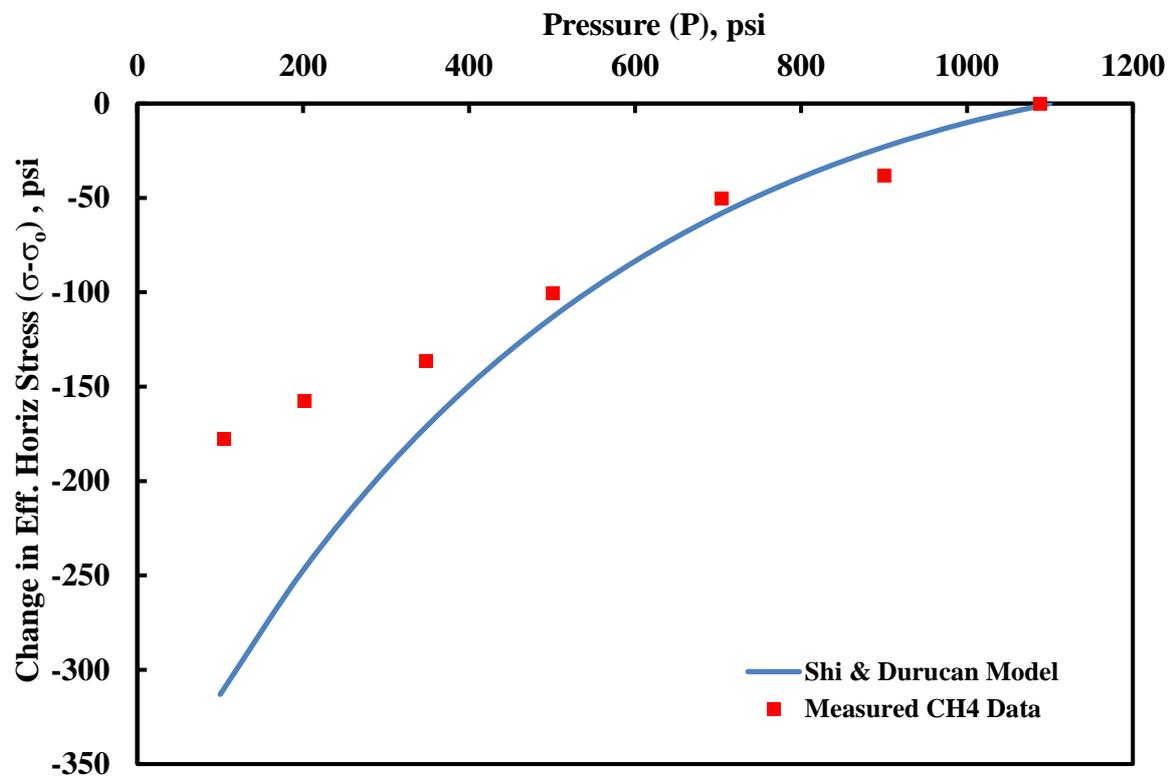
Figure 4-6: Measured and modeled change in eff. horizontal stress with methane depletion (Constant E)
