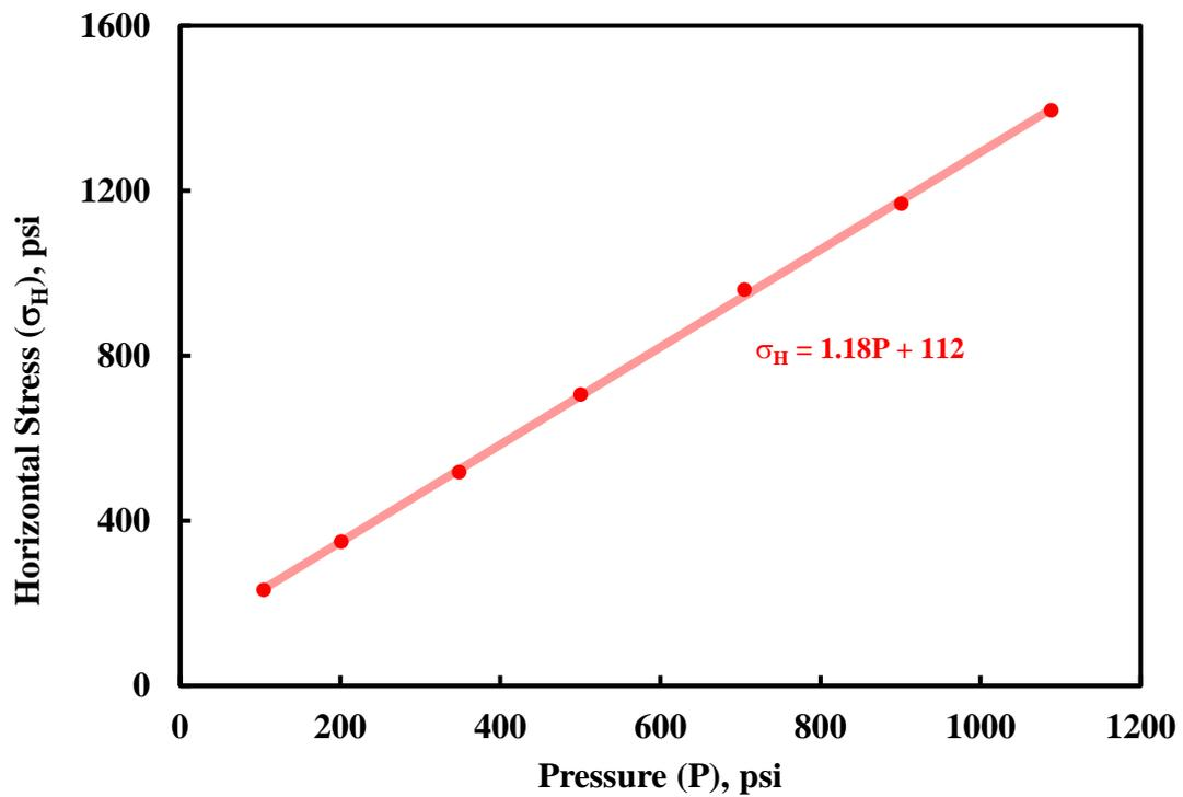
Figure 4-2: Variation in horizontal stress with methane depletion
