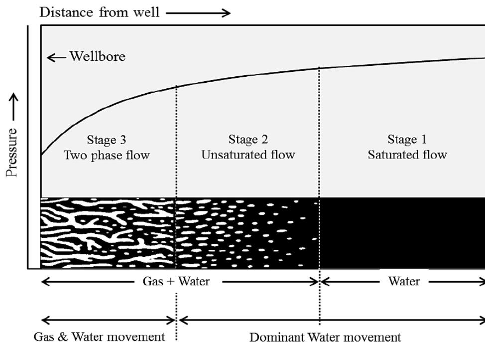
Figure 1-2. Different stages of CBM flow associated with water production (McKee, 1987)
