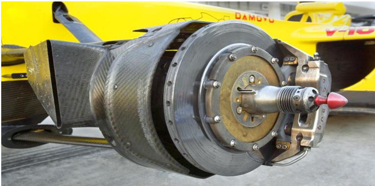
Figure 4-3: Formula1 brake disk made of carbon -carbon composites [15].
