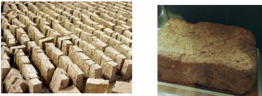
Figure 1-1: Composite bricks made out of straw and mud [17].
