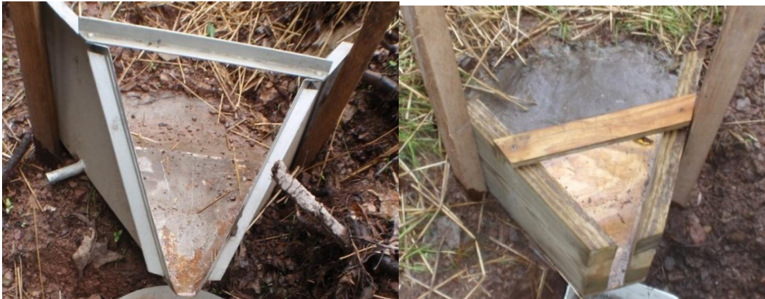
Figure 5. A pre-fabricated metal flume (left) and a constructed wooden flume (right).
