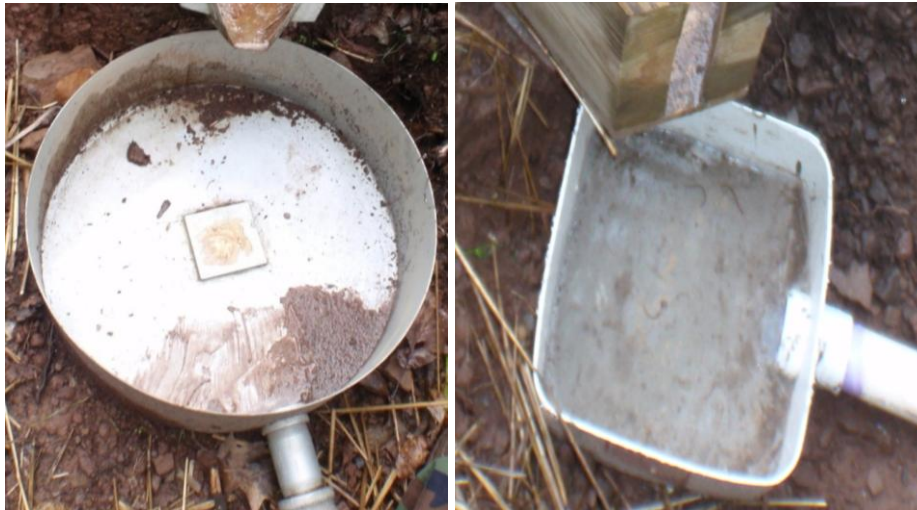
Figure 6. A pre-fabricated metal pan (left) and a constructed plastic pan (right). The flume outlet is at the top of each photograph, and the pipe leading to the tanks is shown at the bottom of the left photograph and on the right of the right photograph.
