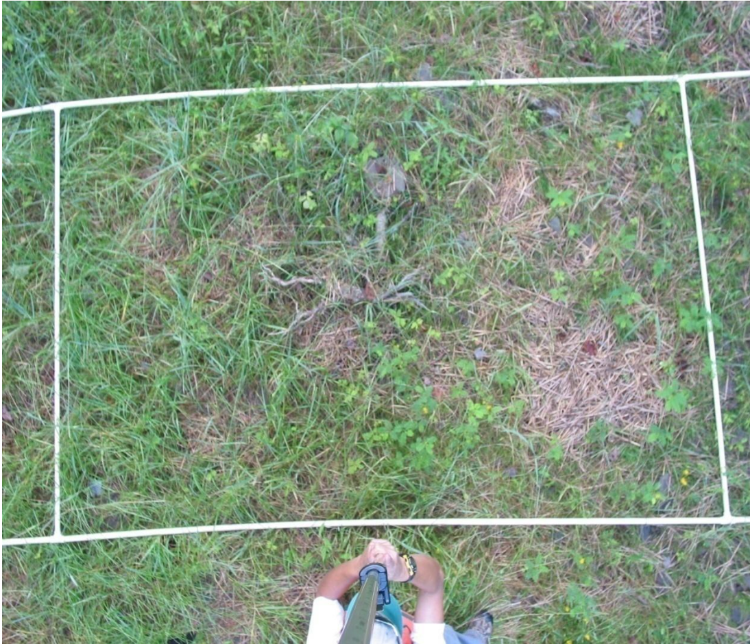
Figure 11. PVC frame used to photograph vegetative cover. The camera was mounted at the top of the pole shown in the bottom of this photograph.
