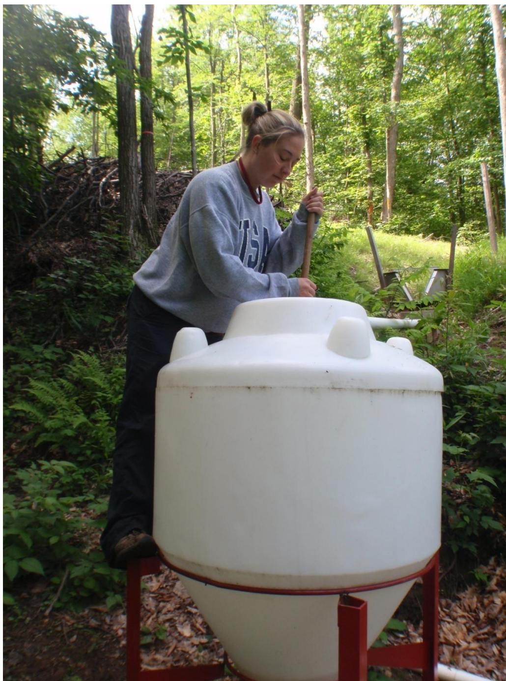
Figure 8. The contents of the tank were re-suspended by stirring prior to sample collection.
