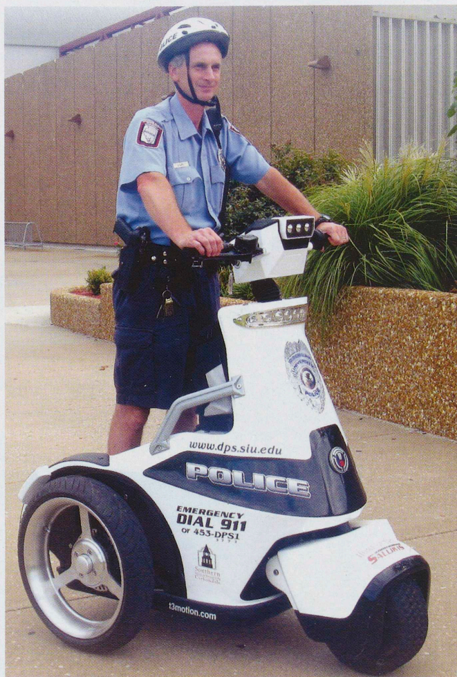
Jamie Lipe, an officer at Southern, shows off the department's T3 Motion all-electric personal patrol vehicle. The environmentally friendly three-wheel vehicle will allow officers easier access to some areas on campus, and features a top speed of 25 mph, a zero-turn radius, and costs about 10 cents per day in electricity.
