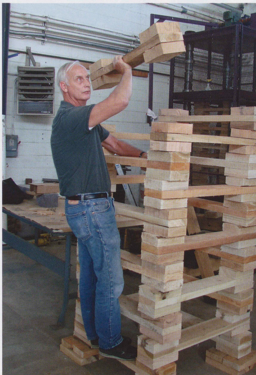
Pulliam demonstrates the ease with which miners can handle the new support system.
