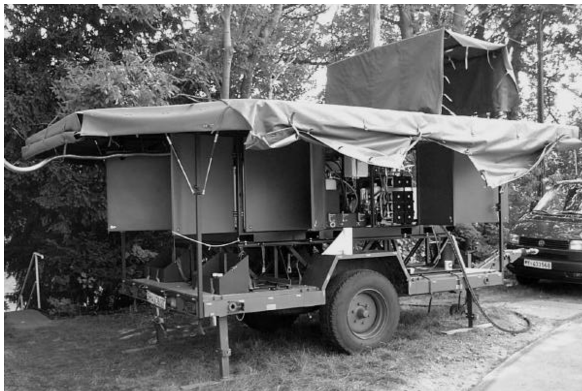
Figure 1: Photography of the mobile drinking water purification unit Kärcher WTC 1600 GT at the field site near the Teltowkanal in September 2000.
