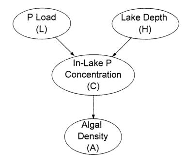
FIGURE 2. Graphical representation of a probability network for the phosphorus loading model.
