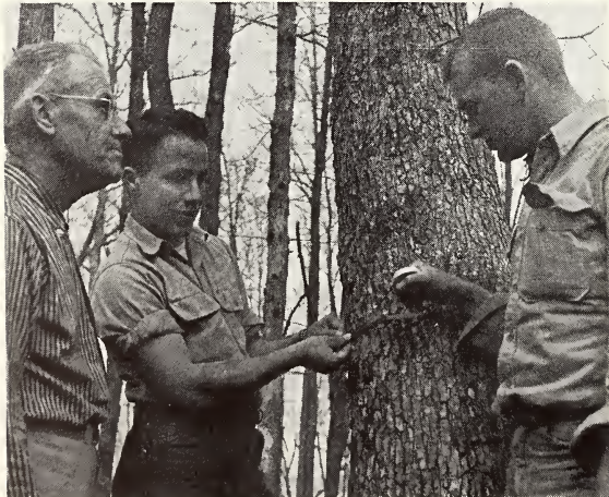
Measuring the diameter of a forest tree with a special steel tape is part of the field experience of forestry students in determining its saw-timber volume.
