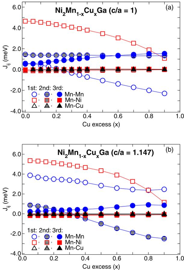
FIG. 2. *Ab initio* magnetic exchange interactions of  $\text{Ni}_2\text{Mn}_{1-x}\text{Cu}_x\text{Ga}$  for the (a) cubic ( $c/a = 1$ ) and (b) tetragonal ( $c/a = 1.147$ ) phase as a function of the Cu excess  $x$ . Here the lines with open (line filled, and filled) symbols are interaction in the first (second, and third) coordination sphere, respectively. The circle (triangle, and square) symbols denote the Mn-Mn (Mn-Cu, and Mn-Ni) interactions, respectively.
