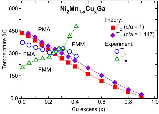
FIG. 4. Theoretical and experimental  $T - x$  phase diagrams for  $\text{Ni}_2\text{Mn}_{1-x}\text{Cu}_x\text{Ga}$ . Theoretical Curie temperatures for the austenitic and martensitic phases are calculated using mean-field approximation. Here,  $T_C$  and  $T_m$  are the Curie temperature and the temperature of martensitic transformation, FMM (PMM) and FMA (PMA) are the ferromagnetic (paramagnetic) martensite (austenite), respectively. Experimental data are taken from Ref. 28.
