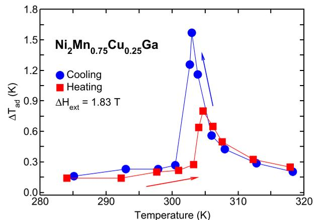
FIG. 1. Adiabatic temperature change  $\Delta T_{ad}$  measured for a Ni<sub>2</sub>Mn<sub>0.75</sub>Cu<sub>0.25</sub>Ga alloy upon heating (squares) and cooling (circles) in the vicinity of the magnetostructural transition. The solid lines are a guide for the eyes.
