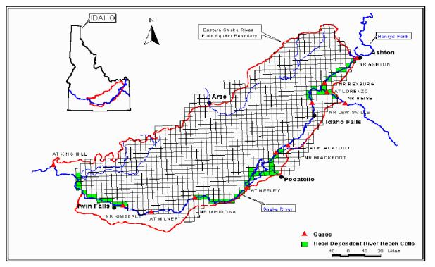
Figure 1 Map of East Snake Plain Aquifer groundwater model area with model grid cells
