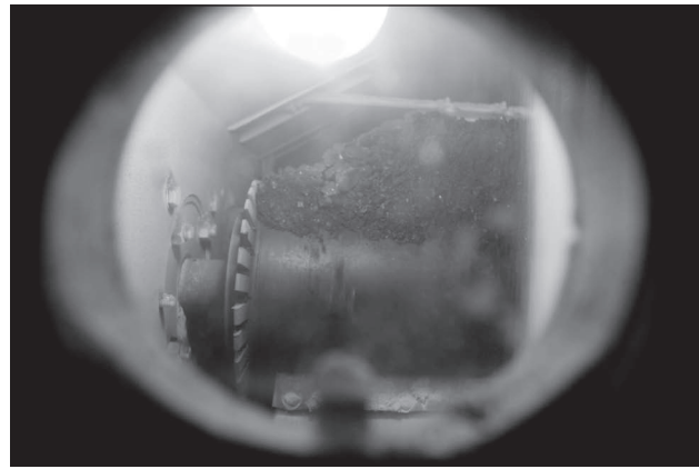
During the coal handling process, the coal is broken up in the crusher and mixed with crushed limestone to absorb sulfur gases. JASON JOHNSON DAILY EGYPTIAN
