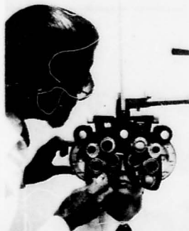
PHOROPTER —this highly accurate instrument is used by the doctor to further refine your prescription
