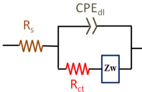
Fig. 2. Randles equivalent circuit for CNLS data fit.
