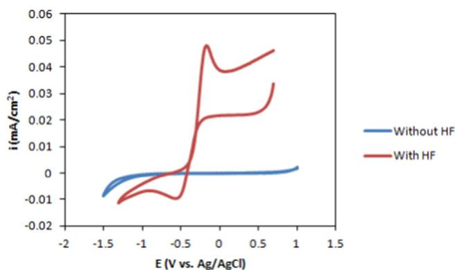
**Fig. 4.** Cyclic voltammogram of bare degenerate Si in an electrolyte containing 200 mM KSCN, 50 mM PBS buffer, and 5.0 mM  $\text{K}_3\text{Fe}(\text{CN})_6/\text{K}_4\text{Fe}(\text{CN})_6$  at pH 7.3, with and without 10 mM HF.
