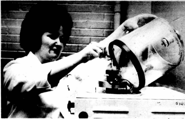
Judith Murphy, director and researcher of the University's Center for Electron Microscopy, freeze-dries a piece of kidney tissue before placing it in the scanning electron microscope. At right, Lorenzo
