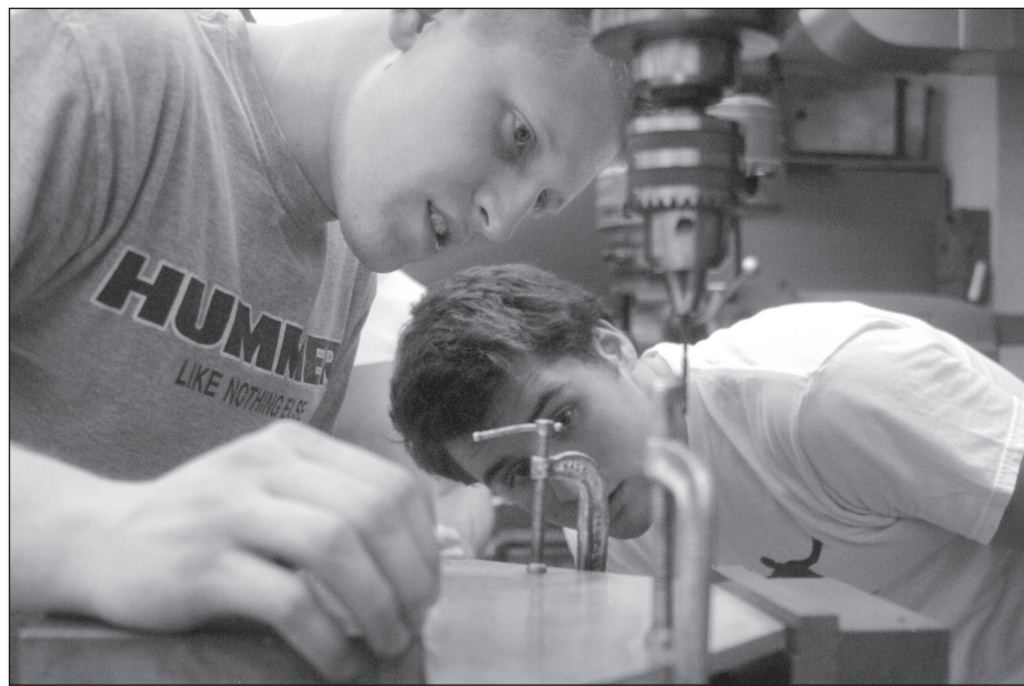
Tyler Madding, a senior from Decatur studying industrial technology, marks drill points on several pieces of metal while Lee Peck, a sophomore studying mechanical engineering, looks on. The metal plates will soon be combined using rivets and will shape the body of the mechanical engineering robot.
