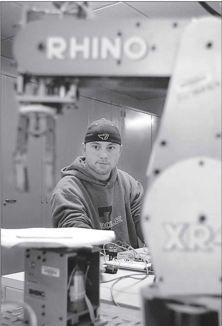
Using wires attached to his forearms, Jim Ehrenstrom, a senior in electronic systems technology from Pinckneyville, watches as he moves the arms of the Rhino XR4. Ehrenstrom is part of a project to develop robots that respond to muscle flexes. In roughly 15 years, the technology will give amputees almost full use of a robotic limb, he said. Timothy Krajcir, a 63-year-old man from Allentown, Pa.
