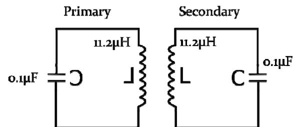
Figure 5. Parallel Resonant Coils
