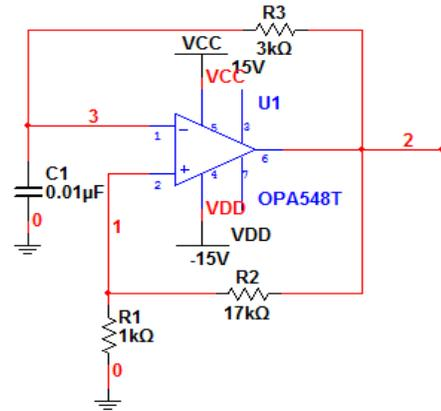
Figure 3. Square-Wave Oscillator
