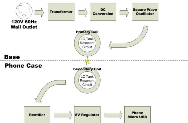
Figure 1. Block Diagram of a Wireless Power Adapter
