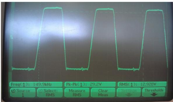
**Figure 9. Square-Wave Generator Output**
