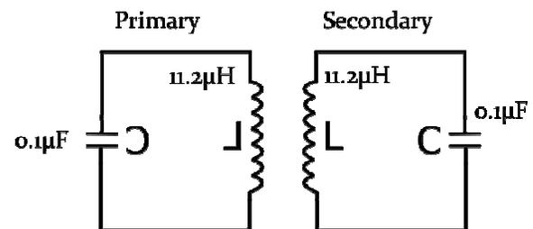
Figure 5. Parallel Resonant Coils
