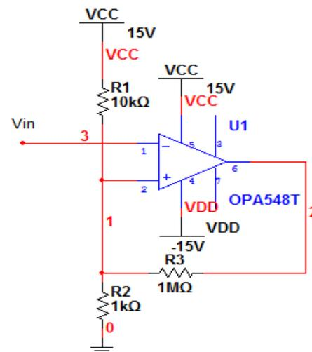
Figure 6. Schmitt Trigger
