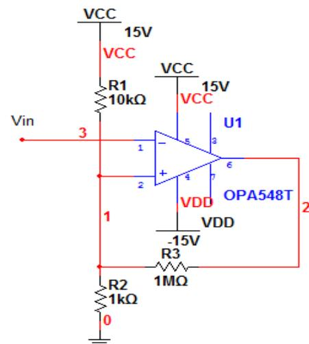
Figure 6. Schmitt Trigger
