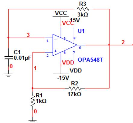
Figure 3. Square-Wave Oscillator
