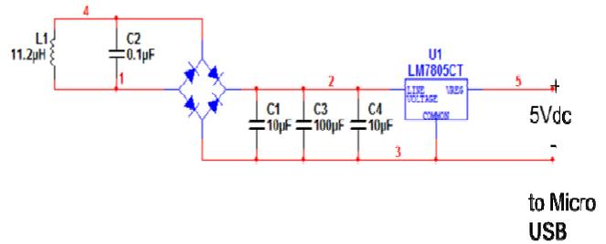
Figure 8. Secondary Circuit
