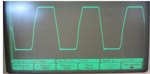
**Figure 10. Schmitt Trigger Output**
