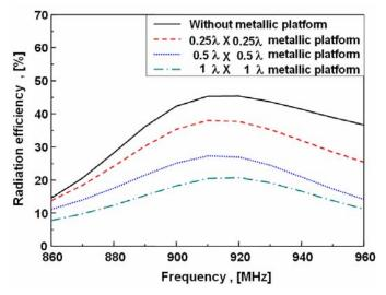
Fig. 4.4 Simulated radiation efficiency for different sizes of metallic platforms
