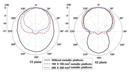
Fig. 4.6 Measured radiation patterns with different sizes of metallic platforms
