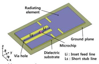
Fig. 4.7 Structure of the compact patch-type tag antenna
