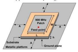
Fig. 3.5 Microstip patch antenna mounted on the metallic platform
