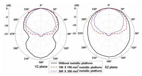
Fig. 4.11 Measured radiation patterns with different sizes of metallic platforms
