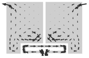
Fig. 4.3 Surface current distribution of balanced-type microstrip patches
