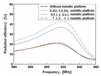
Fig. 4.9 Simulated radiation efficiency for different sizes of metallic platforms
