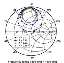
Fig. 3.6 Impedance characteristic with varying the size of the metallic platform
