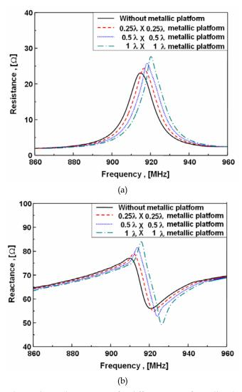
Fig. 4.8 Simulated impedance characteristics for different sizes of metallic platforms
