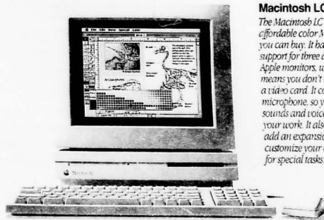
Processor: 68020 Speed: 16 MHz Memory: 2-10 megabytes Expansion slots: One
