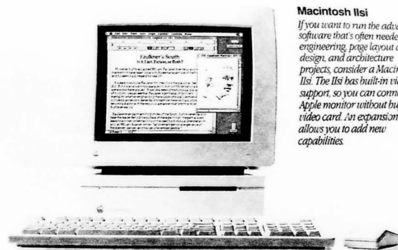
Processor: 68030 (optional 68882 math coprocessor) Speed: 20 MHz Memory: 2-17 megabytes Expansion slots: One
