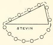
The different way in which Galileo handles the problem of Stevinus marks the beginning of the new Science in which rest is regarded as virtual velocity. When a weight hanging perpendicularly supports a double weight resting on an incline which is double the length of the perpendicular, Galileo sees in the phenomenon one weight tending to descend to the Earth at a certain rate and a double
