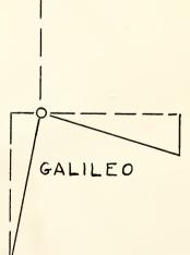
from the long arm and four times the weight depends from the short arm. The position is one of equilibrium and the equilibrium is illustrated by the equality of two triangles two sides of which measure the masses and the spaces which they cover in equal times.
