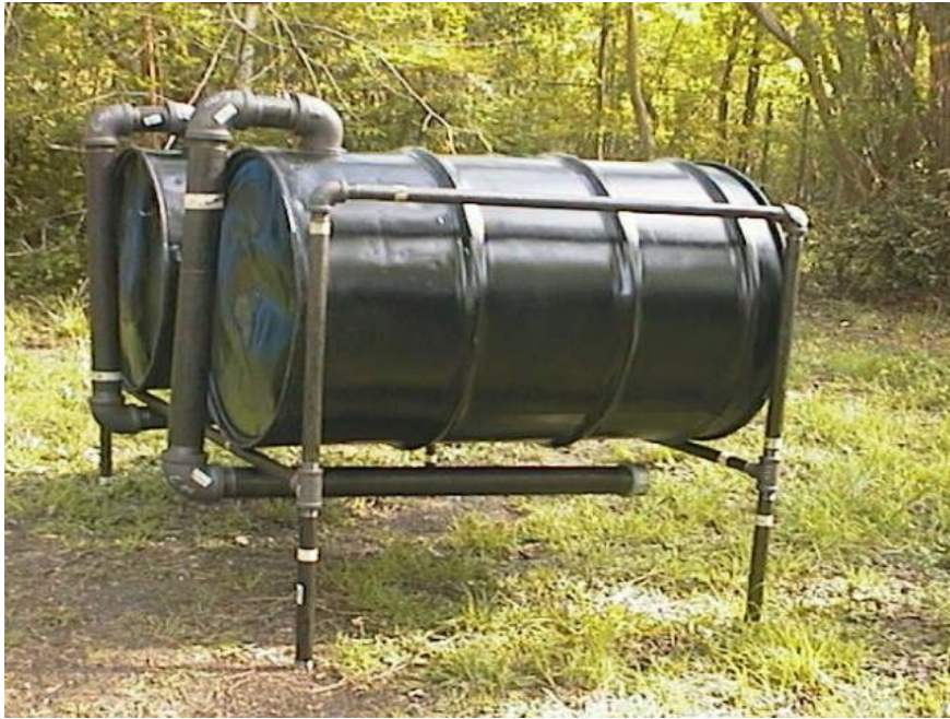
Figure 8. 55-gallon drum kilns. Source: Katanabuilders.com.
