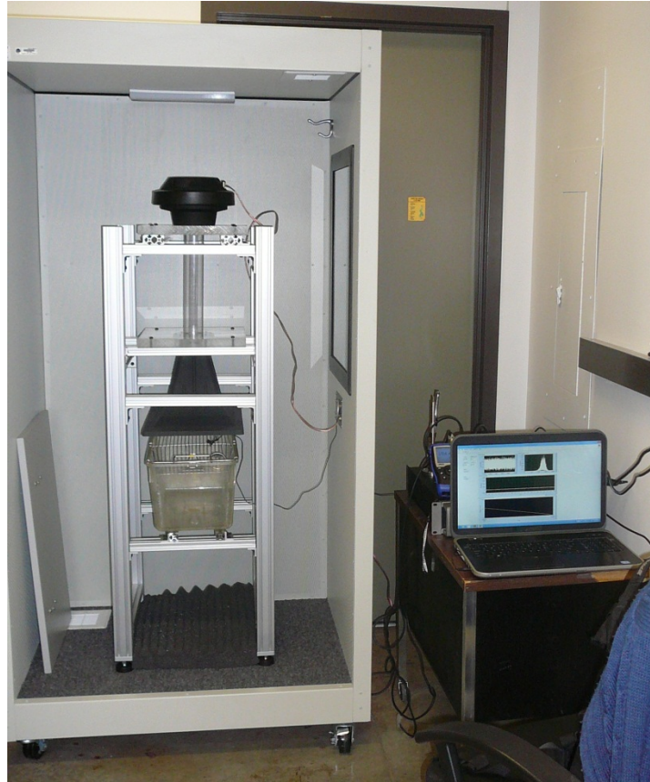
Figure 4: Noise generation system assembled at the SIU School of Medicine
