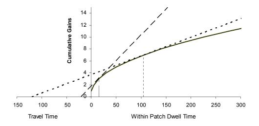
**Figure 1.** Cumulative gain as a function of within patch residence time. The two lines represent two travel time requirements. The short-dashed line and the dashed line represent a 120 s and a 20 s travel requirement, respectively. Optimal switch point is determined by drawing a line from the required travel time tangent to the cumulative gain curve.
