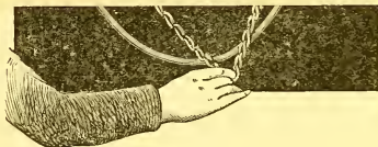
THE CATENARY, OR CURVE FORMED BY A HANGING CHAIN.
