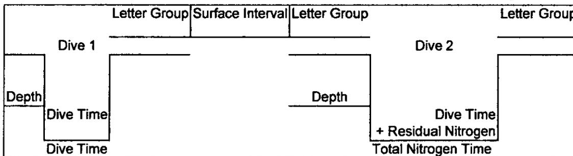
more than one repetitive dive, the same procedure would be used for the third and subsequent profiles. Where the NAUI tables give specific amounts of residual nitrogen in the body at the end of the dive, the NiTek Plus does not. Instead, it shows a digital gauge of nine bars. The greater the number of bars filled at the end of the dive, the greater the amount of residual nitrogen calculated to still be in the body.
