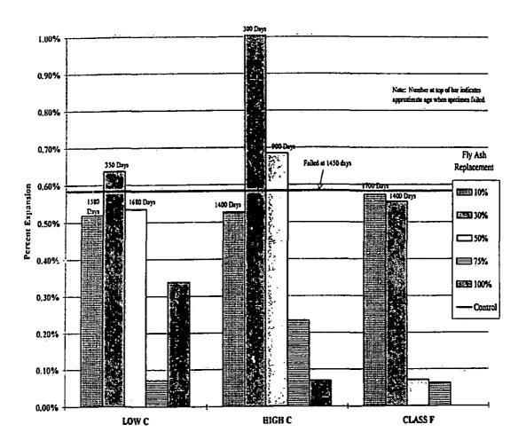
Figure 12. - Expansion of fly ash mixtures with 424 lbm/yd of cementitious materials at about 1650 to 1750 days (accelerated test).
