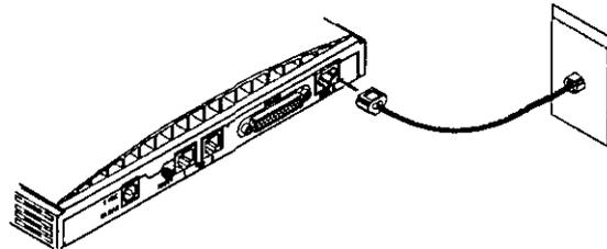
The diagram above shows the proper connection for the modem end of the ISDN cable. Instead of hooking to a telephone jack with the other end of the ISDN cable, as you probably would be doing in a real-life situation, you will instead be connecting to the ISDN simulator.
