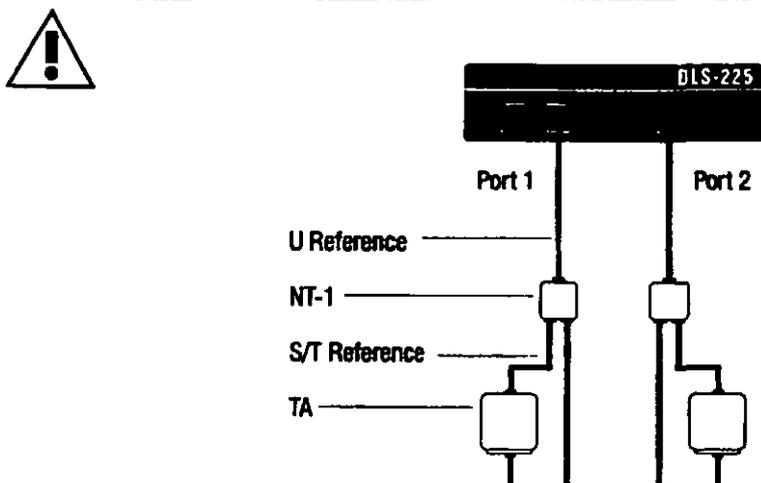
Figure 3 S/T interface operation
