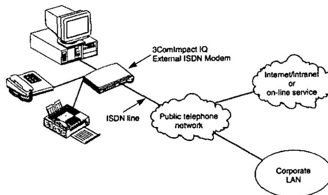
The 3C882 modem is designed to transmit data at speeds of up to 128 Kbps in its standard configuration. Transmission rates of up to 230.4 Kbps are possible with the use of hi/fn® compression and a high-speed serial port.
