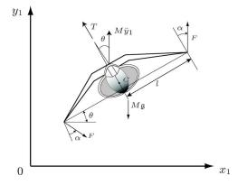
Fig. 1. Forces acting on the aircraft.
