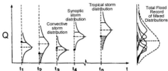
**Figure 2.** Schematic diagram depicting likely probability distributions for peak discharge events ( $Q$ ) arising from different hydroclimatic causes at various times,  $t$ . Based on an analysis of 40 years of peak flows in the southwestern United States (see Hirschboeck, 1988 and Hirschboeck et al., 2000).
