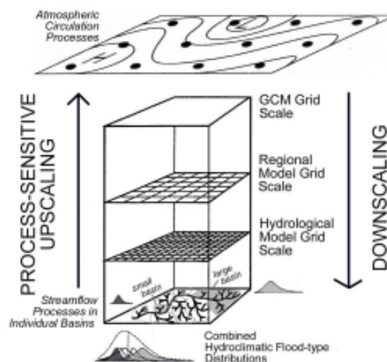
**Figure 1.** Traditional downscaling (right arrow) and process-sensitive upscaling (left arrow). The two approaches are complementary and when used together can provide a more comprehensive assessment of the relationship between atmospheric circulation and hydrologic response.
