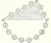
Illustrating proof of the law of the inclined plane. The whole string of balls is in equilibrium; cut away the lower part, and the balls on the sides still remain in equilibrium; hence the powers on the sides are as the number of the balls, or as the lengths.
