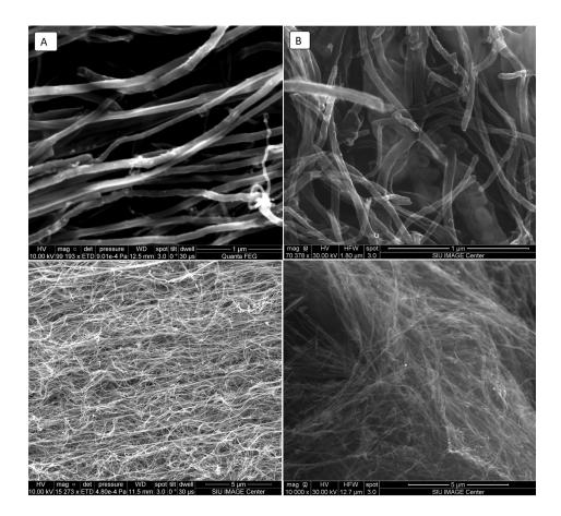
FIG. 1. SEM images of CNT without Gd (a) and CNT+Gd (b).
