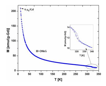
FIG. 4. MvT of CNT-Gd composite obtained at applied magnetic field H = 20kG calculated per Gd atom using the results of EDAX analysis (see Table I).
