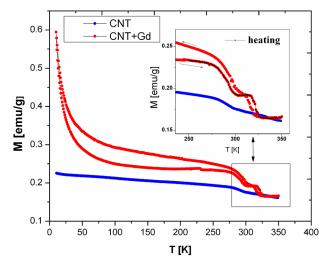
FIG. 3. MvT at 500G for CNT and CNT+Gd.
